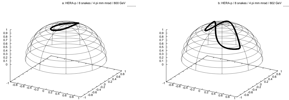
Figure 2: The \hat{n} -vector for the 4\pi mm mrad ellipse at 800 GeV (left) and 802 GeV (right).
