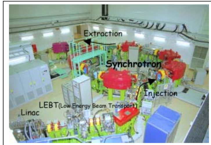
Figure 4.7: The medical synchrotron installed in the Tsukuba Proton Treatment facility of Japan. The requirements of these accelerators for the appropriate medical treatments are very stringent, and there is a significant amount of development needed to optimize their size and operability for use in a clinical environment.
