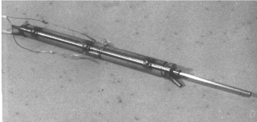
FIGURE 4: 30 cm-long superconducting undulator with period 10 mm and the axis field \sim 5 kG. Diameter of thin wall stainless steel chamber is 6 mm, wall thickness 0.1mm.
