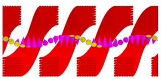
Figure 1: 3d OPERA multiwire model of the undulator. Cones represent the magnetic field vector.
