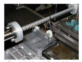
Figure 4: Undulator winding on a lathe.
