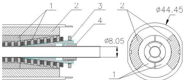
Figure 3: Details of design. 1–Iron yoke, 2–Copper collar, 3, 4–trimming Iron nuts. Inner diameter of Copper vacuum chamber is 8mm.
