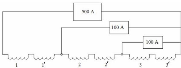
Figure 6: Electrical scheme of feeding the undulator windings. In 12mm-period undulator coils 1 and 1' are located closer to the Iron helix, coils 2 and 2' are the next, 3 and 3' are in the middle of coil (Indicated current is approximate).
