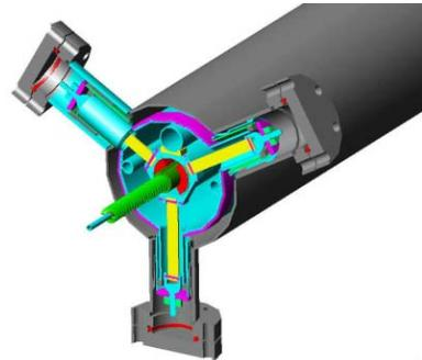
Figure 2: Details of cold mass support. Outer tube diameter is 5 inch.
