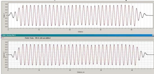
Figure 9: Longitudinal field distribution for 12 mm period undulator at 200 A and 250A. Here the left axis shifted inside undulator (graph below). One can see the difference at the left.
