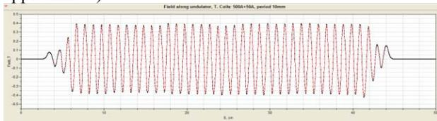
Figure 7: Longitudinal field profile for 10-mm period undulator measured with Hall probe. Current in main PS 500A, additional PS running at 50A.  $K=0.36$  in regular part. Variation of field is picks is from 0.399T to 0.309 T.
