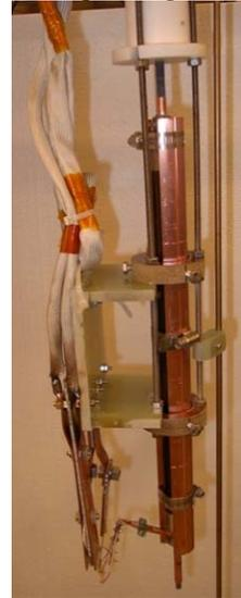
Figure 5: Undulator cold mass installed into Dewar vertically for measurements with Hall probe. Undulators with 10 and 12-mm period look identically. Stick at the right is a liquid Helium level meter. Hall probe holder is running through central hole.
