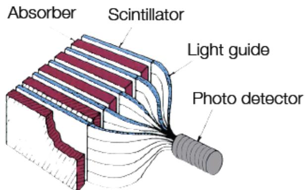
Scintillators as active layer; wave length shifter to convert light
