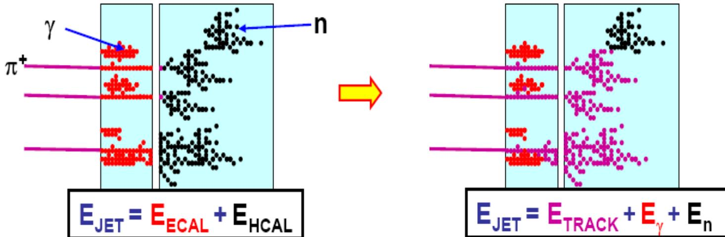
**PFLOW calorimetry = Highly granular detectors (CALICE)
