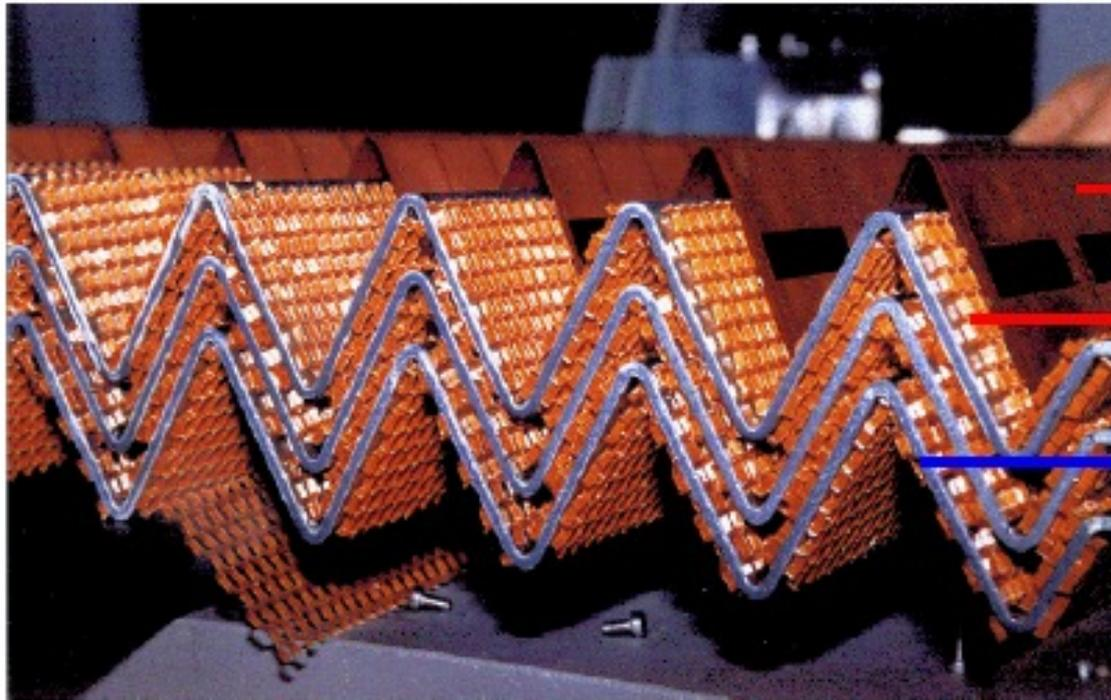
Cu electrodes at +HV
