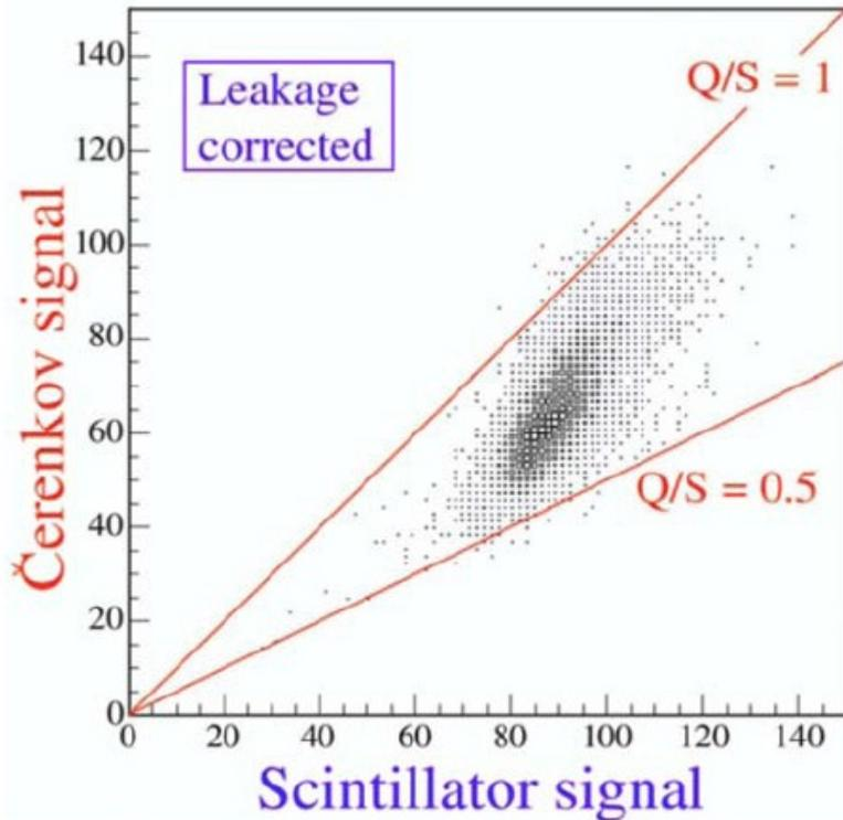
$Q/S < 1 \rightarrow$  ~25% of the scintillator signal from pion showers is caused by non-relativistic particles, typically protons from spallation or elastic neutron scattering
