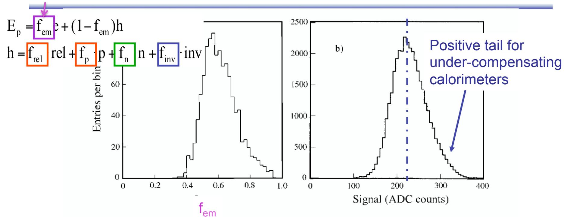
FIG. 4.44. The distribution of the fraction of the energy of 150 GeV  $\pi^-$  showers contained in the em shower core, as measured with the SPACAL detector (a) [Aco 92b] and the signal distribution for 300 GeV  $\pi^-$  showers in the CMS Quartz-Fiber calorimeter (b) [Akc 98].
