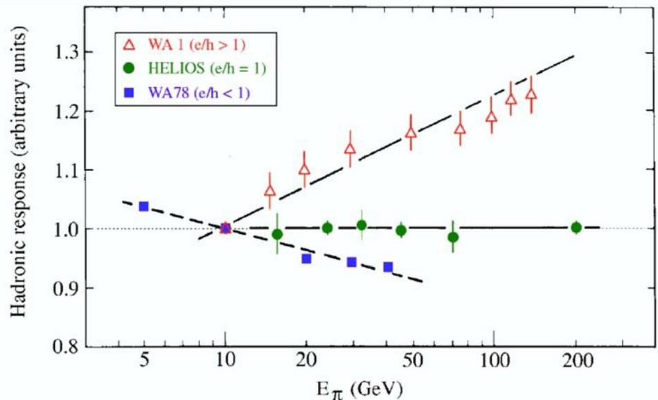
FIG. 3.14. The response to pions as a function of energy for three calorimeters with different  $e/h$  values: the WA1 calorimeter ( $e/h > 1$ , [Abr 81]), the HELIOS calorimeter ( $e/h \approx 1$ , [Ake 87]) and the WA78 calorimeter ( $e/h < 1$ , [Dev 86, Cat 87]). All data are normalized to the results for 10 GeV.
