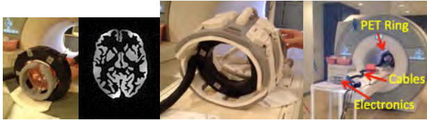
Fig. 17. Preliminary study of the approach to use standard flexible RF coils to minimize the effect of active PET on MRI. Imaging with the 3T Flex Large flexible RF coil with coil inside PET ring (far left). A flexible coil placed outside the ring in a complementary imaging study (middle right). The experimental setup with the PET ring placed inside the 3 Tesla Siemens MRI (far right). An image of a brain phantom filled with water with a 3T Flex RF coil placed between the brain phantom and the PET ring (middle left). The PET system was fully powered during imaging.
