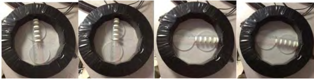
Fig. 8. Set of six 1mm point Na22 sources placed in a line with 20, 20, 20, and 10mm center-to-center spacing. The line of sources was placed in four positions to probe the spatial resolution and linearity response (left-to-right: Position 1,2,3,4).
