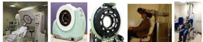
Fig. 1. Displayed here is some of the relevant prior art. From left to right: Siemens' HRRT, Photo Diagnostic Systems' NeuroPET/CT imager; Philips Digital Photon Counting's TOF PET; the PET-Hat; and the WVU Helmet_PET (different, yet similar to the ring described here) in non-MRI, upright form.
