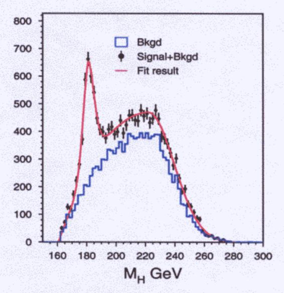
Signal is fitted with assymetric gaussian
