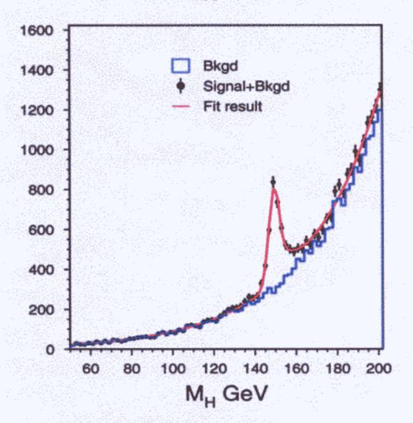
Signal is fitted with assymetric gaussian
