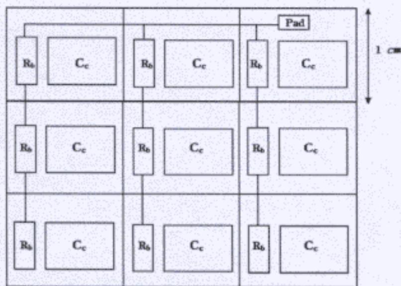
The arrangement of the Silicon wafer, for the example of 3x3 diode wafer.
