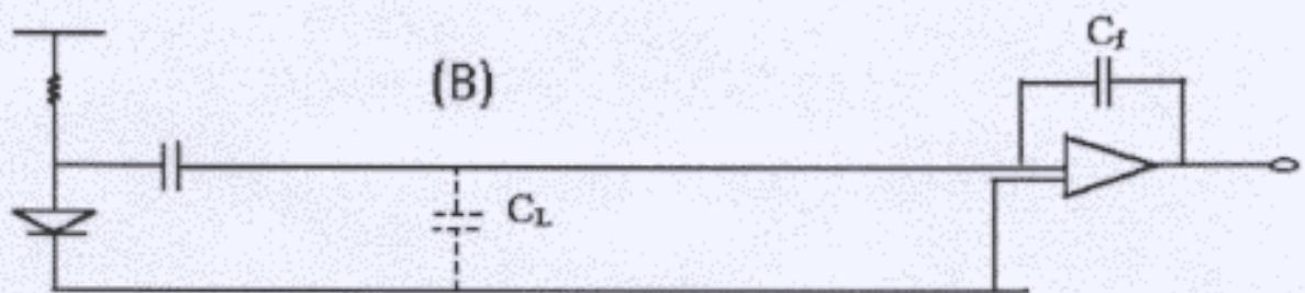
The two possible solutions for the coupling capacitance and resistance.
