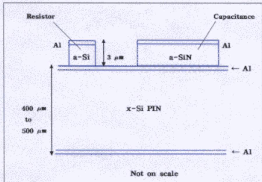
Schematic view of the PIN diode with the amorphous silicon deposited.
