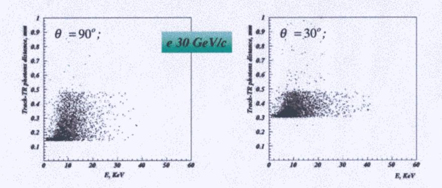
Two dimensional plots of distance between charge particle track and TR photons vs absorbed TR photons energy
