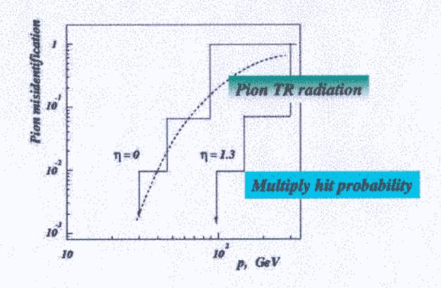
Pion rejection factor of 6 to 100 or greater can be achived over a wide range of momentim up to 90 GeV/c for electron detection efficiency of more 90%;
