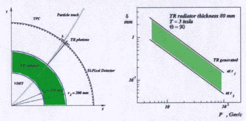
The value of separation between charge particle track and TR photons for present geometry
