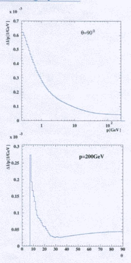
Design resolution reached for  $\theta > 20^{\circ}$  and  $p > 30 \,\text{GeV}$
