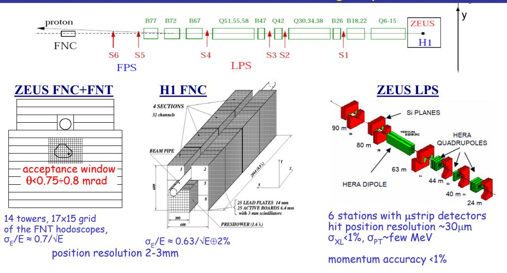
Acceptance limited by beam apertures and detector size  $p_T$  resolution is dominated by  $p_T$  spread of proton beam (50-100 MeV)
