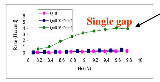
Increase of the noise rate during the irradiation. Nevertheless the value remains below 10 Hz/cm<sup>2</sup>.
