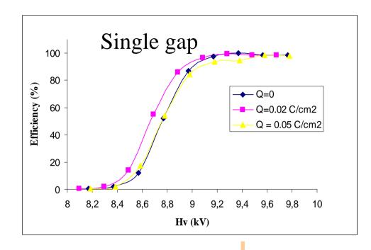
The chamber efficiency in the central region was measured using cosmic muon triggers (measurements # 1, #2, #3)....
