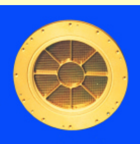
Fig. 5: Detector widow: 1 \mu m polypropylene foil with carbon and lexan coating
