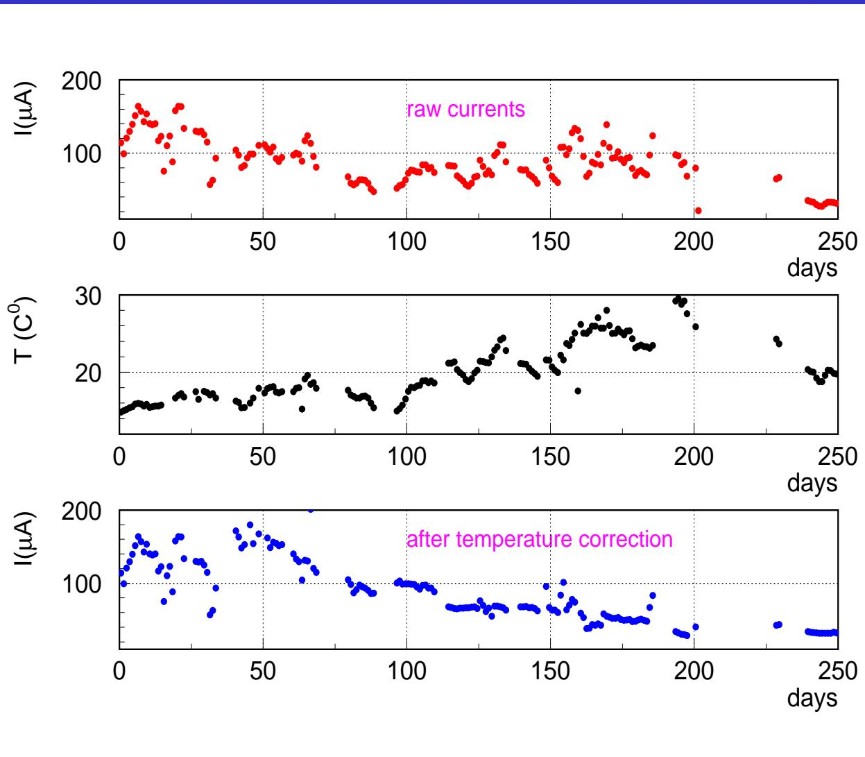
Currents, HV and temperature are continuously monitored
