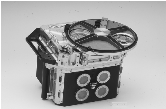
Fig. 2. Integrated Detector. On top of the detector housing is a filter wheel with four positions: open, closed, Boron filter and vacuum door with three calibration sources.
