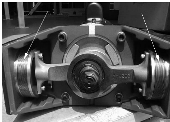
Fig. 8. One of 15 system pumps[22] with cover removed to show steel bellows (arrows).
