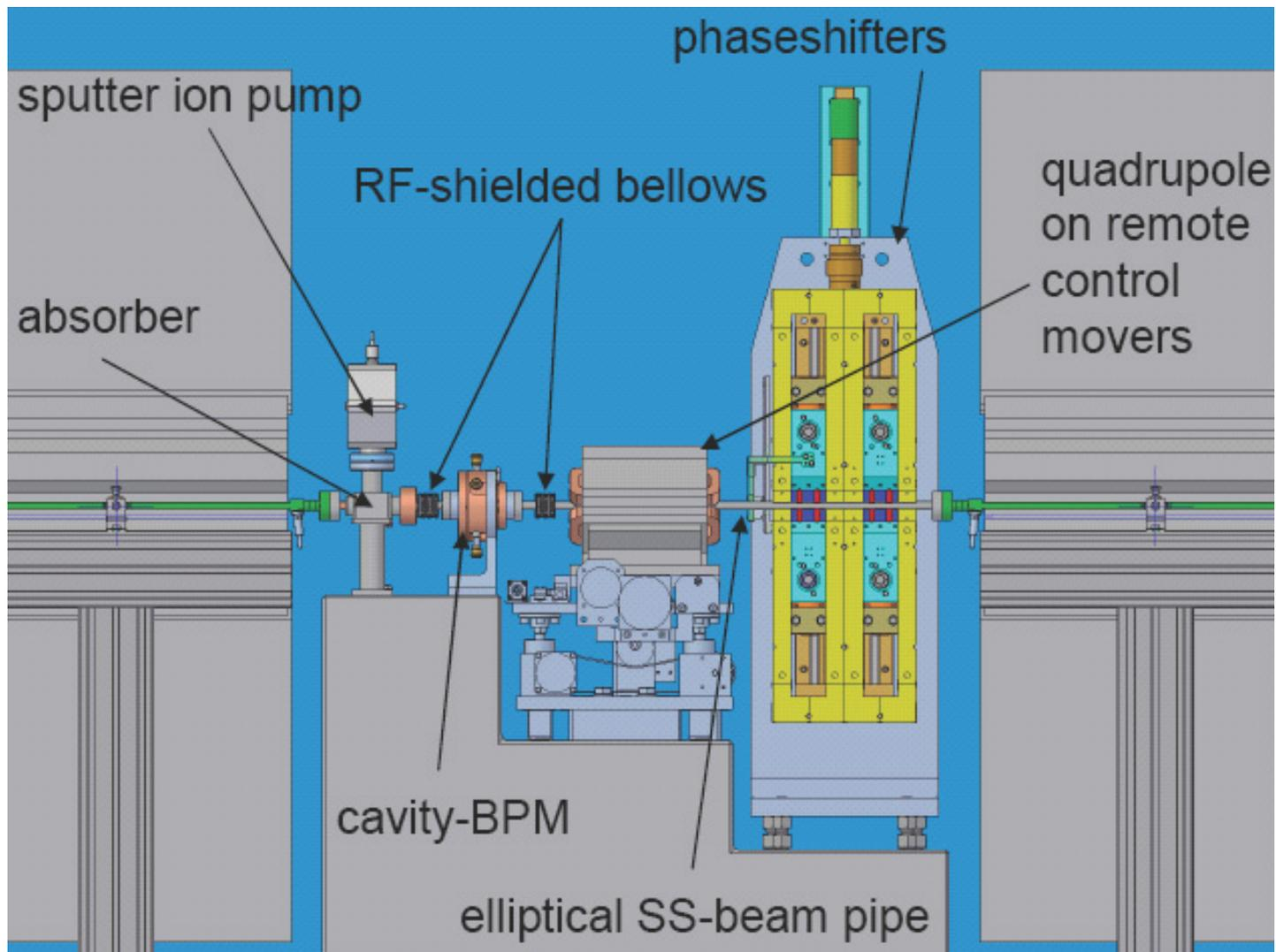
UNDULATOR- CELL(6.1m) = UNDULATOR (5m) + INTERSECTION (1.1m)
