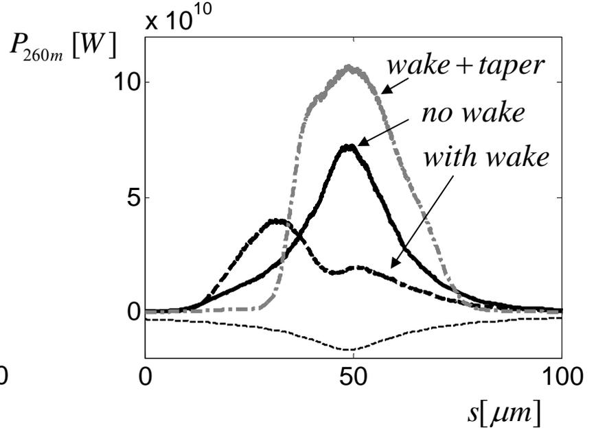
The radiation power in the middle (left) and at the end of the undulator (right)
