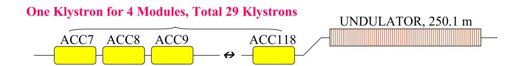
Multi-Klystron before BC2 reduces the jitter sensitivity in ACC234 and ACC39 modules
