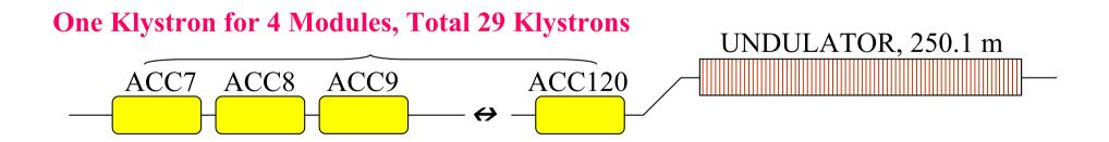
Multi-Klystron before BC2 reduces the jitter sensitivity in ACC334, ACC39, and ACC56
