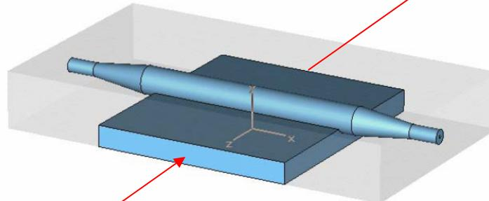
Coaxial cable impedance matching model
