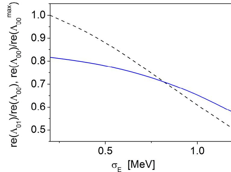
Ratio of the field gain of the first azimuthal mode TEM\_01 to the gain of the ground FEL mode TEM\_00 versus rms energy spread in the electron beam (blue curve). Black dashed curve shows relative reduction of the gain of the fundamental TEM\_00 mode. Radiation wavelength is 8 nm, peak current is 1.5 kA, rms normalized emittance is 1 mm-mrad. Focusing beta function is 10 m.
