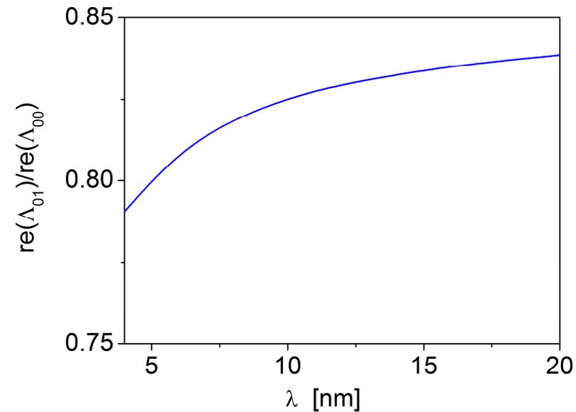
Ratio of the field gain of the first azimuthal mode TEM<sub>01</sub> to the gain of the ground FEL mode TEM<sub>00</sub> versus radiation wavelength. Peak current is 1.5 kA, rms normalized emittance is 1 mm-mrad. Focusing beta function is 10 m.
