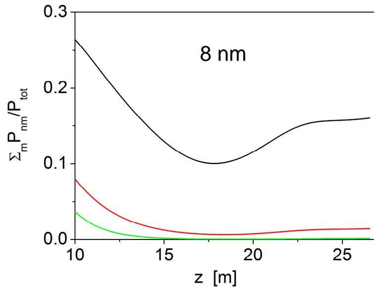
Partial contribution of the higher azimuthal modes of the fundamental harmonic to the total radiation power. Peak current is 1.5 kA, rms normalized emittance is 1 mm-mrad. Black, red, and green curves refer to the modes with  $n = +/- 1$ ,  $n = +/- 2$ , and  $n = +/- 3$ .
