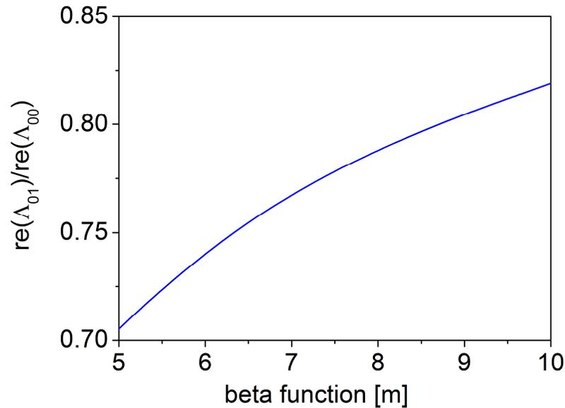
Ratio of the field gain of the first azimuthal mode TEM\_01 to the gain of the ground FEL mode TEM\_00 versus focusing beta function. Radiation wavelength is 8 nm, peak current is 1.5 kA, rms normalized emittance is 1 mmrad
