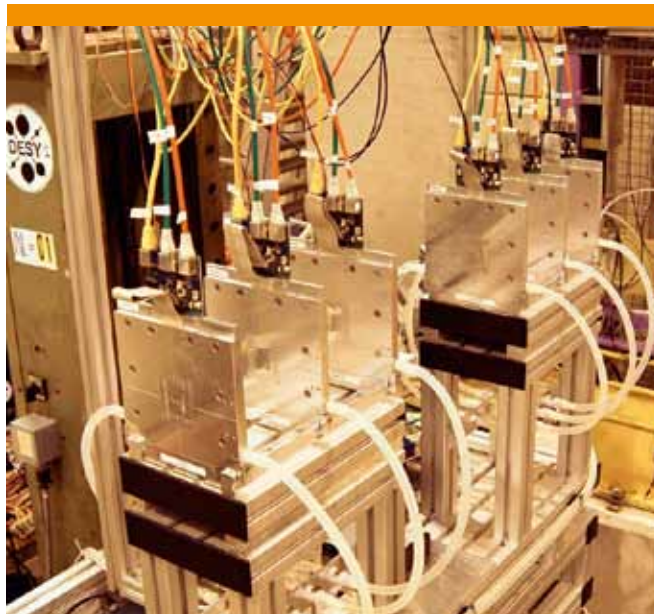
The EUDET telescope installed at the CERN test beam.
