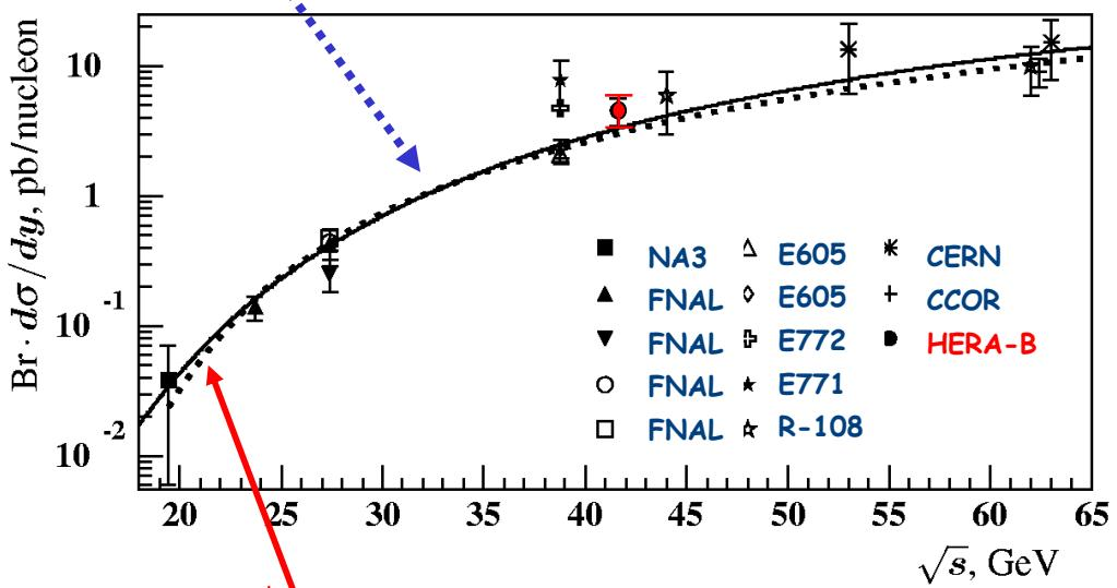
$$Br \times \left. \frac{d\sigma_Y}{dy} \right|_{y=0} (\sqrt{s}) = \sigma_o \exp \left( -\frac{m_o}{\sqrt{s}} \right)$$
