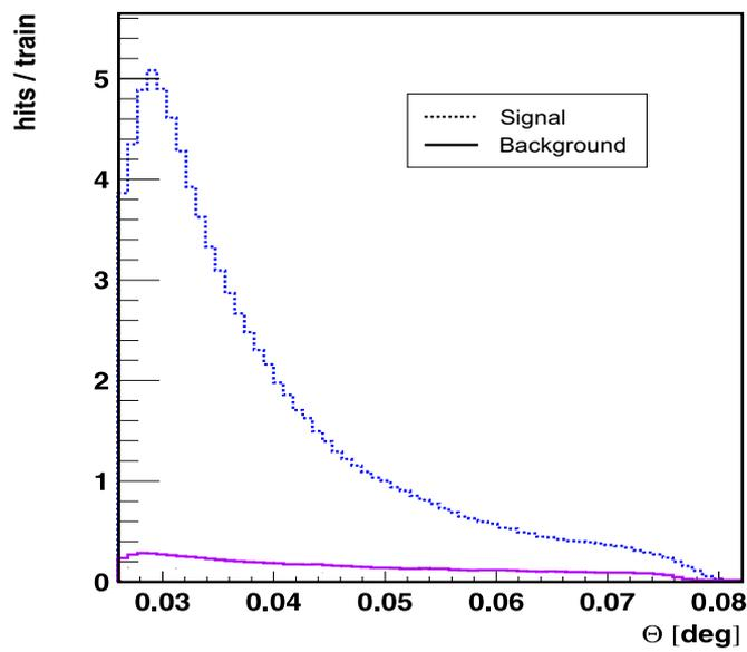
Figure 7: Occupancy in the luminosity calorimeter for signal (dashed line) and background (solid line).
