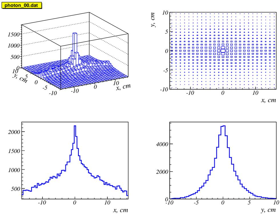
Figure 42: Distributions as seen by the IBS camera from head-on collisions at the IP. Upper left is a plot of positron intensity versus horizontal ( $x$ ) and vertical ( $y$ ) directions transverse to the beamstrahlung beam. Upper right is the the same as seen in the  $x - y$  plane. Lower left and right are projected intensity distributions in  $x$  and  $y$ , respectively.
