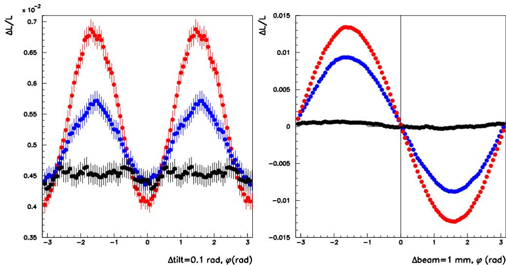
Figure 18: The relative shift on the luminosity as a function of the angle of tilts (left) and the angle of beam shifts (right) for three cases: the detector is aligned on the outgoing beam (black dots); for a 14mrad crossing angle with the alignment on the detector axis (blue dots); the detector is aligned on the detector axis for a 20mrad crossing angle (red dots).
