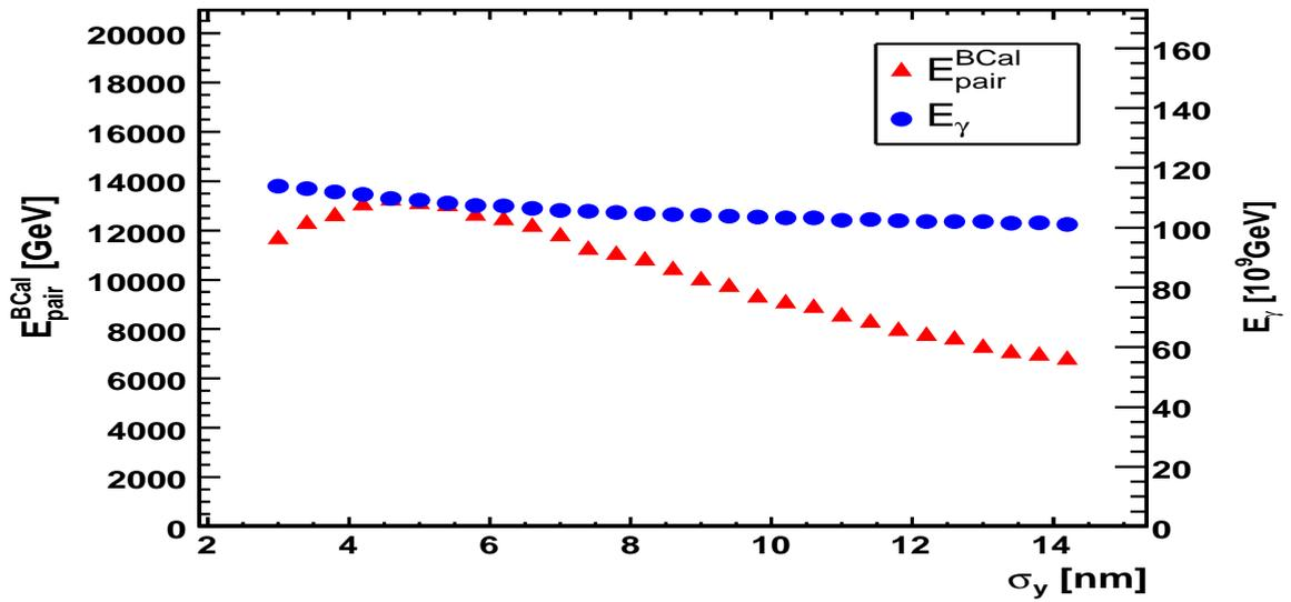
Figure 38: Energy of the gammas (right scale) and the pairs hitting the BeamCal (left scale) per beam crossing as a function of the bunch height (nm).
