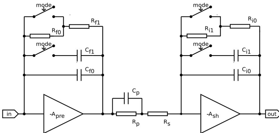
Figure 58: Schematic of preamplifier, PZC and shaper. Switches set to test mode.
