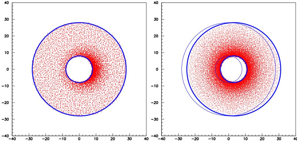
Figure 17: Distribution of Bhabha scattering events for a 20mrad crossing angle ILC. Two cases are shown: the detector is positioned on the detector axis (left) and along the outgoing beam (right).
