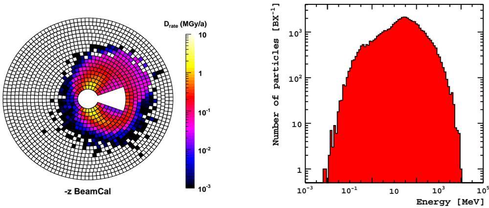
(a) Radiation load as simulated for LDC for 14 mrad, DID field and 100% running time per year.
