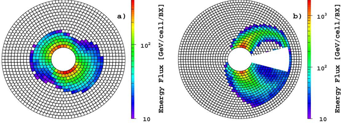
Figure 34: The energy density of beamstrahlung remnants per bunch crossing as a function of position in the  $r - \varphi$  plane at the a) 2 mrad and b) 20 mrad with DID field crossing angles.
