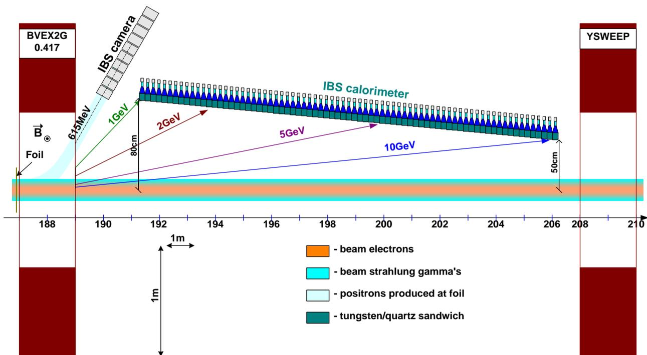
Figure 40: Schematic concept drawing of the Integrated Beamstrahlung Spectrometer (IBS)
