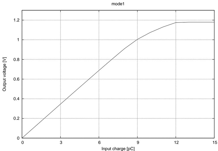
Figure 61: Example of front-end output amplitude vs input charge.
