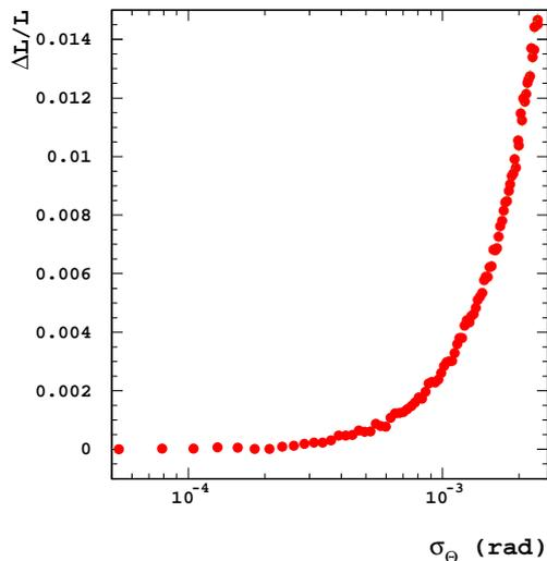
Figure 16: The relative error on luminosity,  $\Delta L/L$ , as a function of  $\theta$  resolution,  $\sigma_\theta$ , calculated using five million Bhabha scattering events for each point.
