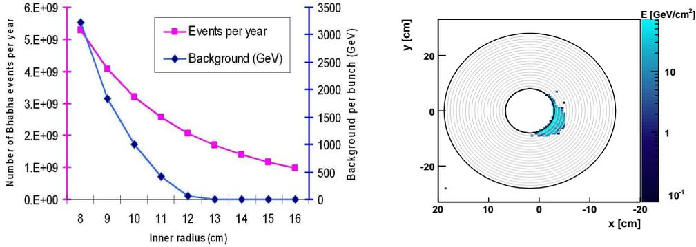
Figure 19: On the left, the background originating from beamstrahlung pairs (blue) and the number of expected Bhabha events per year (pink) as a function of the inner radius. On the right, beamstrahlung pairs hitting the LumiCal. The total amount of beamstrahlung depositions is several TeV. This simulation was done for 20 mrad crossing angle, DID field configuration and a LumiCal position at  $z = 305$  cm. Nominal beam parameters are assumed at a centre-of-mass energy of 500GeV.
