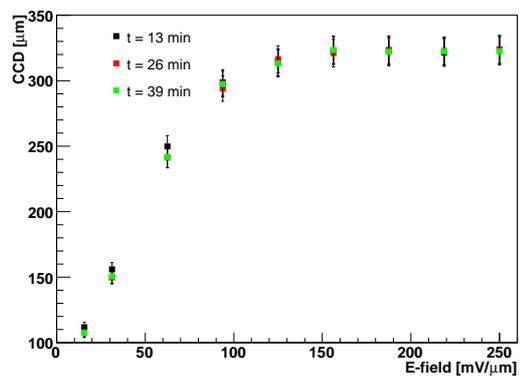
Figure 51: Charge collection distance of sCVD diamond versus electric field.
