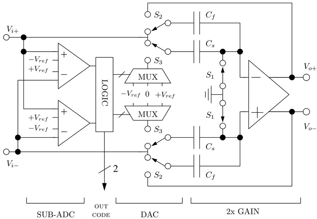
Figure 66: Simplified schematic of a 1.5 bit stage. Switches set to the  $\varphi_1$  phase.
