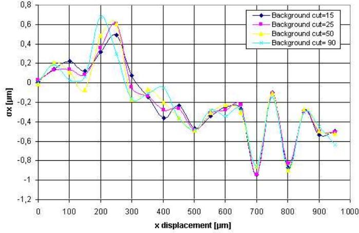
Figure 24: Difference between calculated and real position in x direction.
