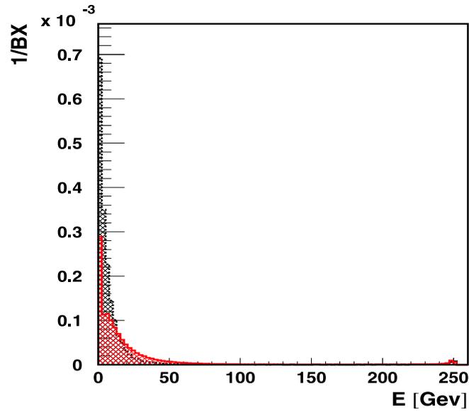
Figure 6: Energy distributions for leptonic (solid line) and hadronic (dashed line) background in the luminosity calorimeter.
