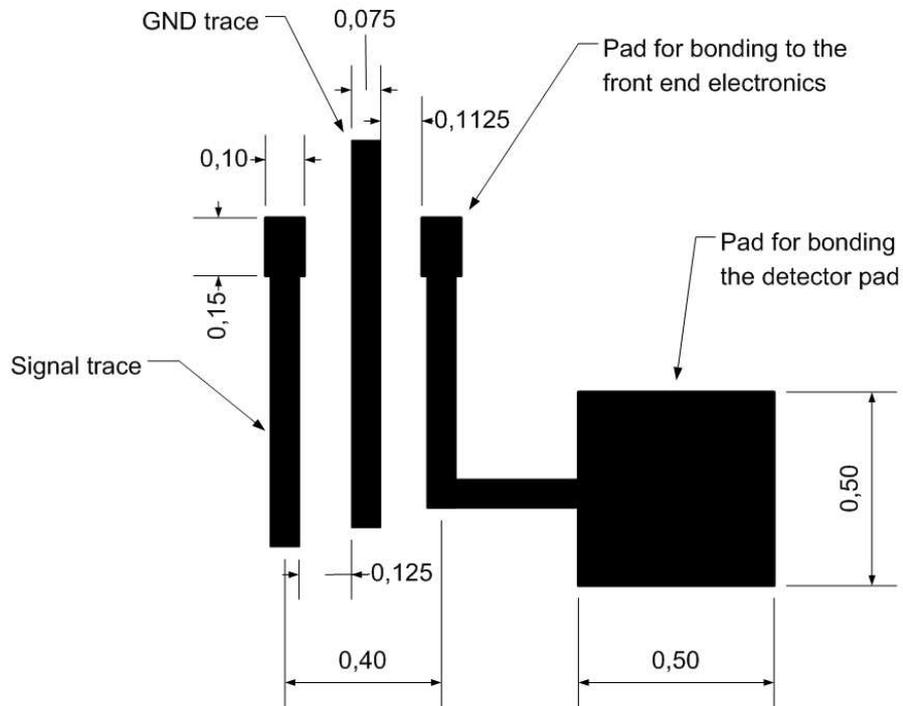
Figure 57: Detailed view of pads and signal traces of the fan-out (all dimensions in mm).
