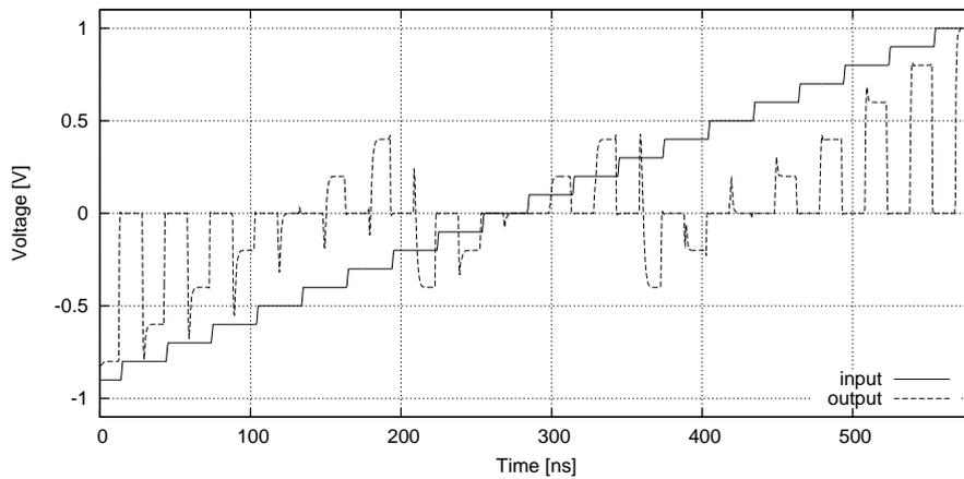
Figure 67: Example of a single 1.5 bit stage output for a staircase function.
