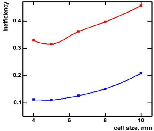
Figure 32: The inefficiency to detect electrons of 200 GeV as a function of the size of the sensor pads. The blue and red curves are obtained for regions of low and high background, respectively.
