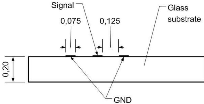
Figure 56: The cross section of the fan-out (all dimensions in mm).
