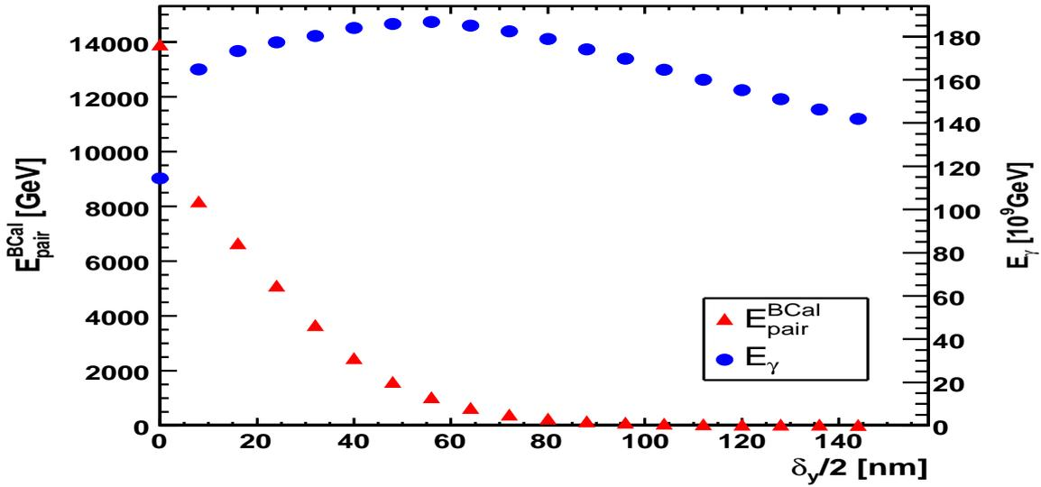
Figure 36: Energy of the gammas (right scale) and the pairs hitting the BeamCal (left scale) per beam crossing as a function of the bunch vertical offset.
