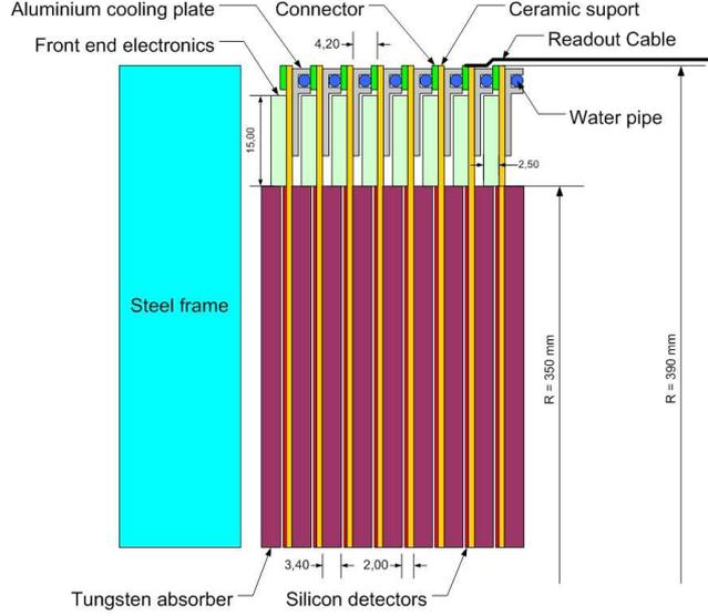
Figure 15: Mechanical design of LumiCal.
