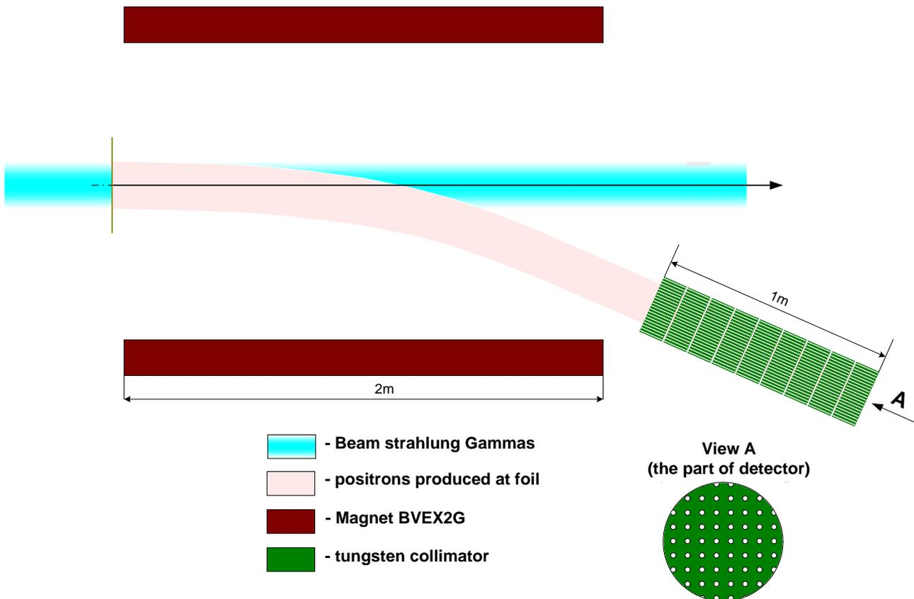
Figure 41: Schematic concept drawing of the IBS camera. The inset shows a sample of the matrix of holes.
