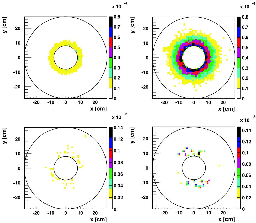
Figure 8: Projection of hits at the front plate of the luminosity calorimeter for leptonic (left) and hadronic (right) background, before (top) and after (bottom) applying the set of isolation cuts (1,2,3).
