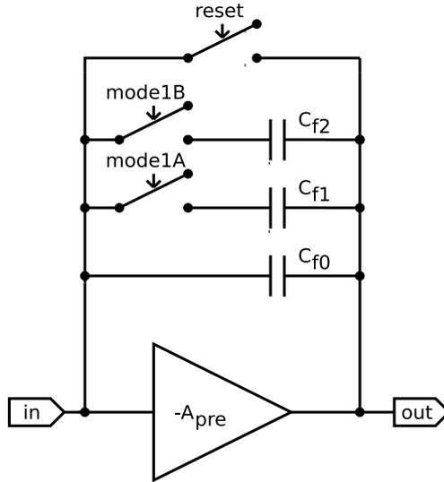
Figure 62: Schematic of preamplifier with reset switch.
