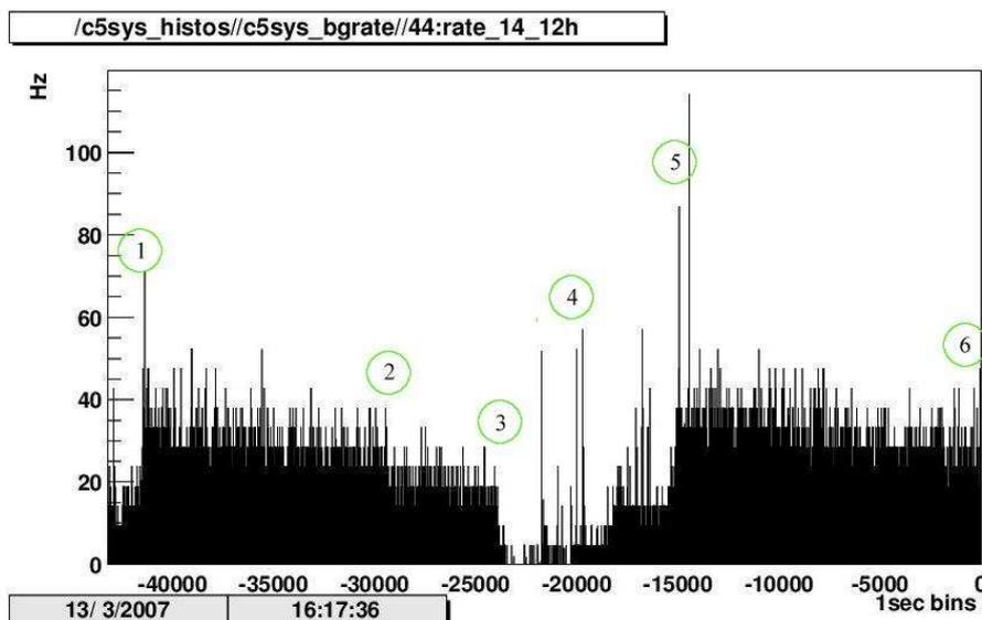
(b) SCVD Diamond beam monitor count rate during 12 h out of the period covered above.
