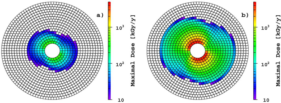
Figure 28: The expected dose in the most exposed longitudinal plane as function of position in the  $r - \varphi$  plane at a) LowQ and b) LowP beam parameter configuration.
