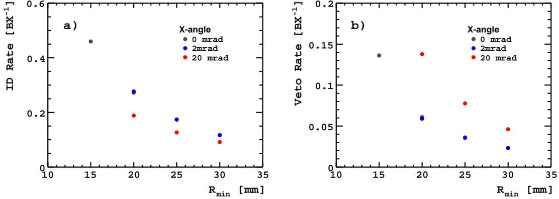
Figure 35: a) Bhabha identification rate and b) Bhabha induced veto rate in the BeamCal as function of the minimal acceptance radius for various crossing angle schemes.
