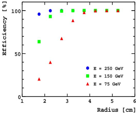
Figure 31: The efficiency to identify an electron of energy 75, 150, 250 GeV as a function of the radius in the BeamCal.
