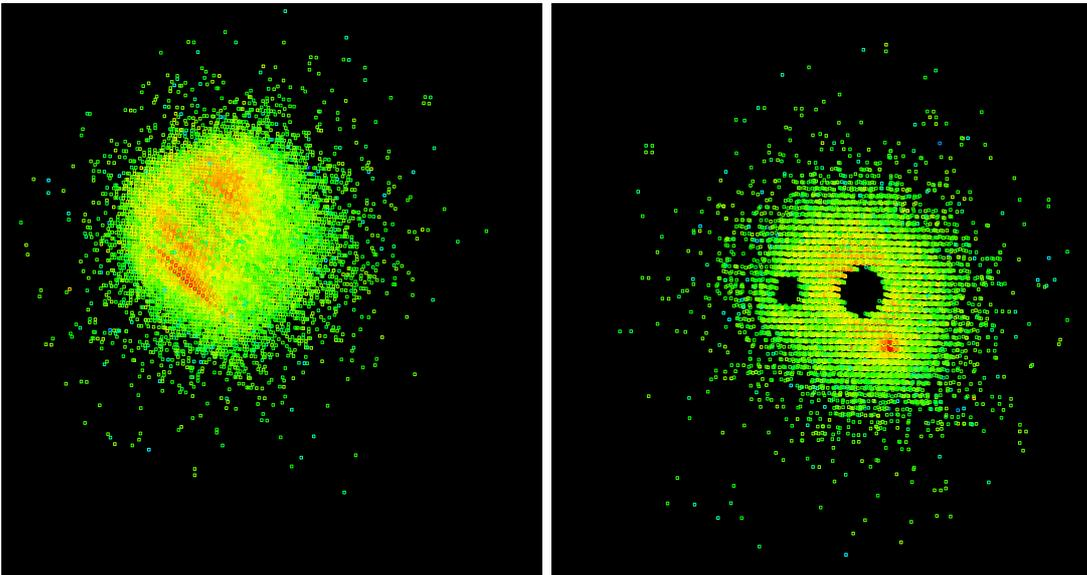
Figure 29: The shower due to the electron from a two photon event of nearly 250 GeV shown overlaid with the beamstrahlung pairs from a random bunch crossing. The figure on the left is the sideview and on the right is the head-on view. The presence of the electron beam exit beam pipe at 7 mrad to the forward direction and the entrance beam hole of the positron beam at -7 mrad are also visible.
