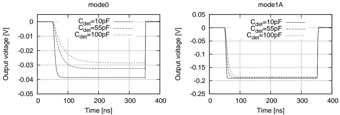
Figure 63: Example of Switched-Reset front-end output in the test mode for 10fC input charge (mode0) and in the physics mode for 1pC input charge (mode1).
