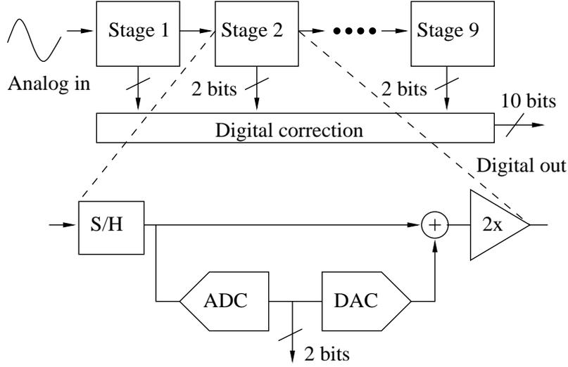
Figure 65: Pipeline ADC architecture.
