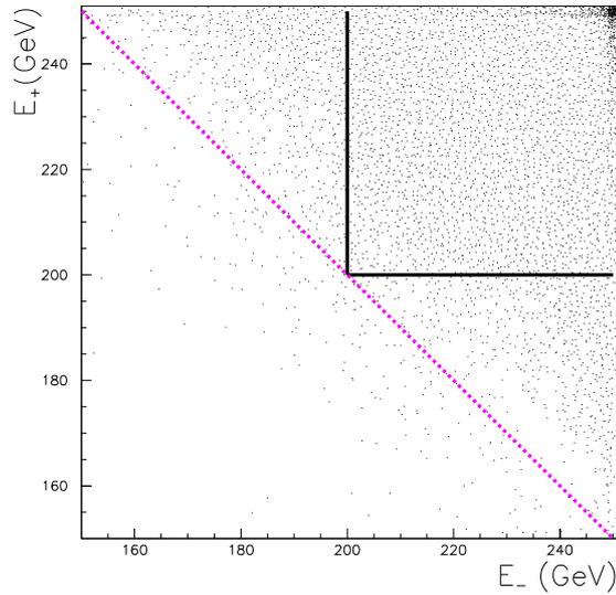
Figure 11: Energy of the positron versus energy of the electron for each final state particle of the Bhabha events passing the angular cuts defined in Equation 2.
