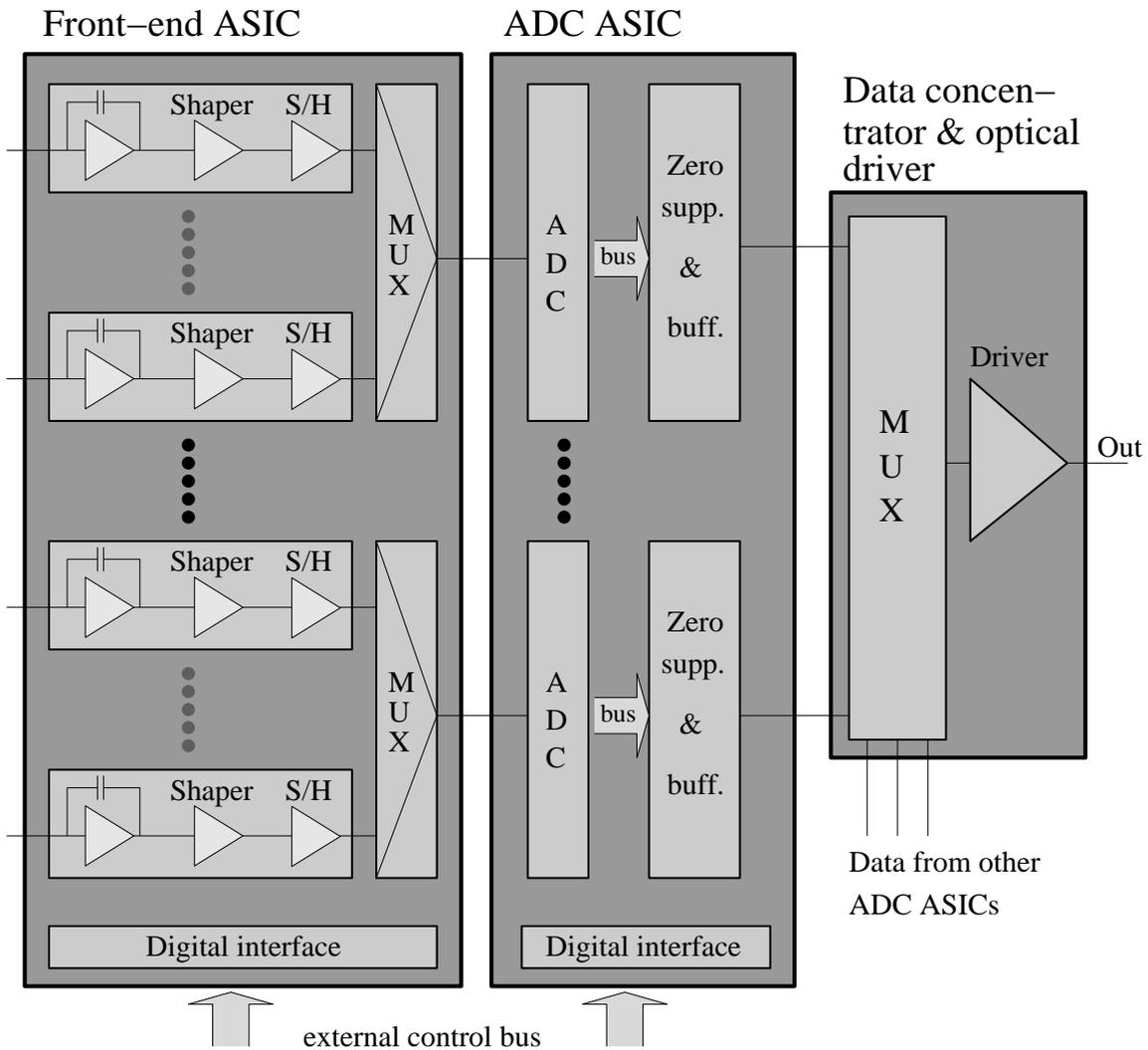
Figure 55: Block diagram of the LumiCal readout electronics.
