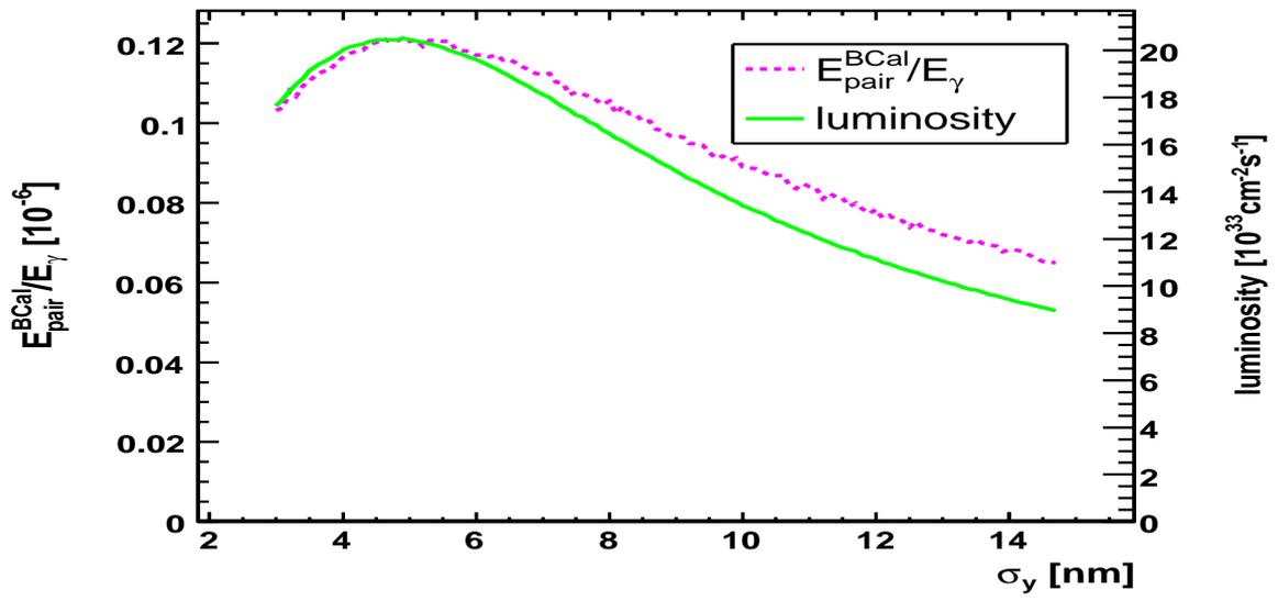
Figure 39: Luminosity (right scale) and the ratio of the pair to gamma energy (left scale) as a function of the bunch bunch height(nm).
