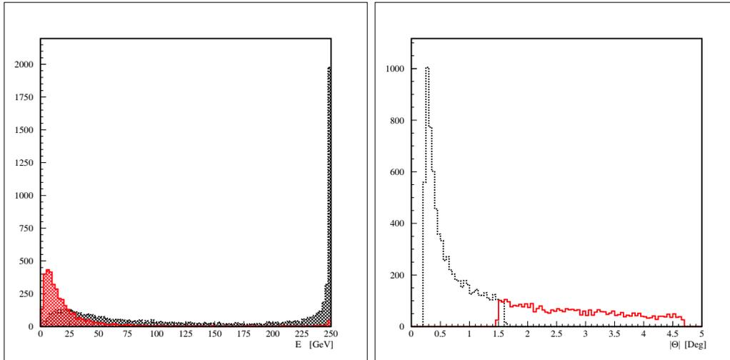
Figure 5: Energy and polar angle distributions of generated particles in the beam calorimeter (dashed line) and luminosity calorimeter (solid line) acceptance region.
