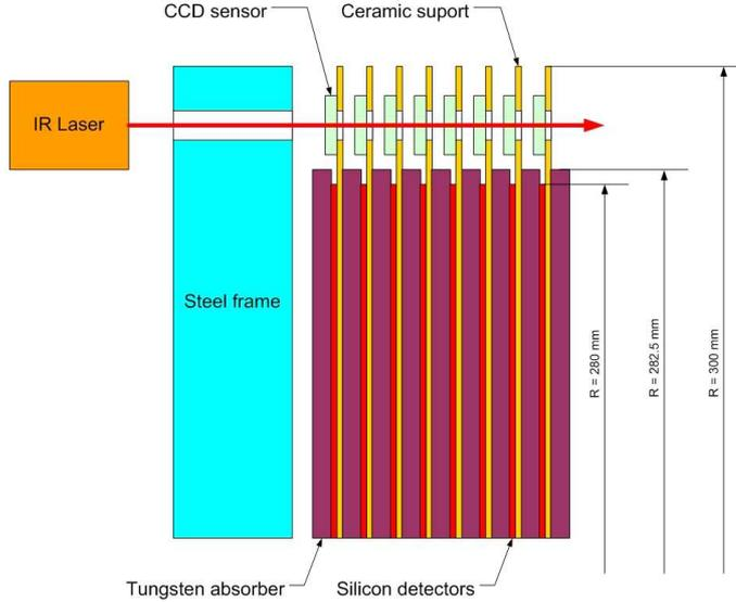
Figure 26: Sensors planes laser alignment using transparent light sensors.
