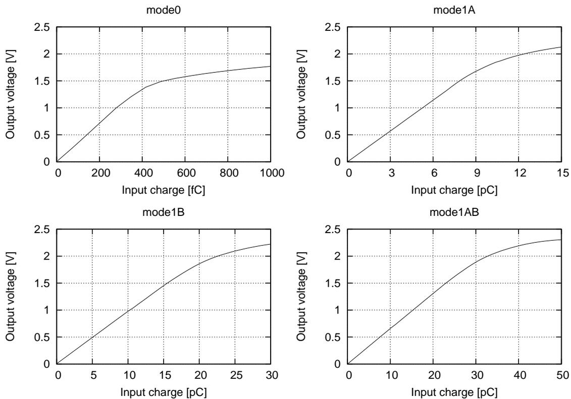
Figure 64: Example of front-end output amplitude versus input charge.
