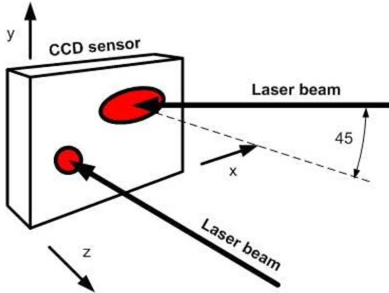
Figure 23: Simplified diagram of two laser beams setup.
