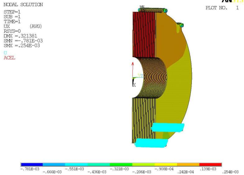
Figure 21: The result of the calculation of the LumiCal deformation when supported over the full length.
