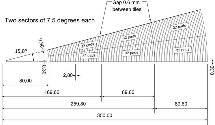
Figure 22: Two azimuthal sectors consist of three silicon tiles.
