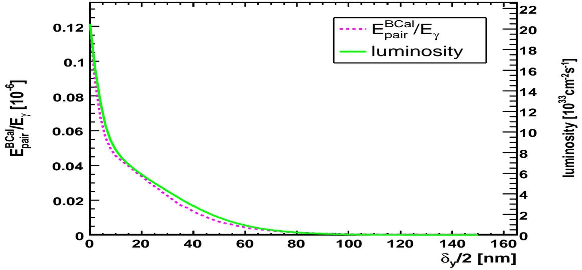
Figure 37: Luminosity (right scale) and the ratio of the pair to gamma energy (left scale) as a function of the bunch vertical offset.
