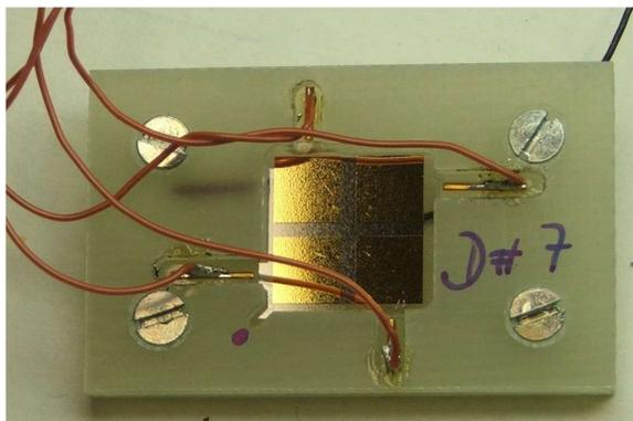
Figure 48: Sample of pCVD diamond with four pads.
