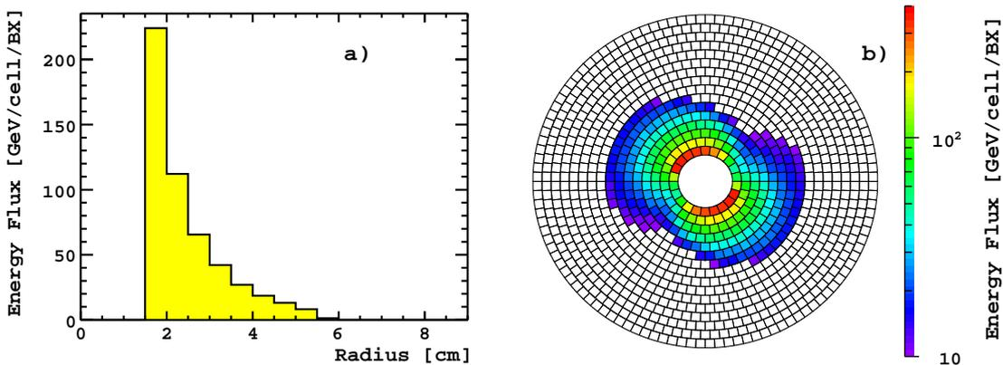
Figure 27: The energy density of beamstrahlung remnants per bunch crossing as a function of a) radius and b) position in the  $r-\varphi$  plane. The centre-of-mass energy is 500 GeV. The maximal value of the density is 350 GeV per cell.
