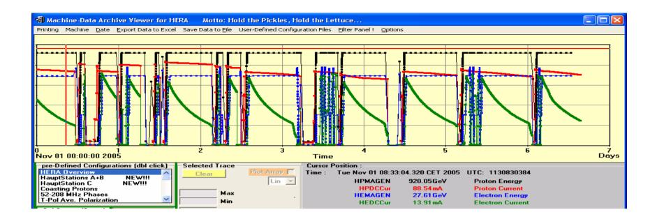
**Beam currents:** Ip =  $87\text{mA} \dots 99\text{mA}$
