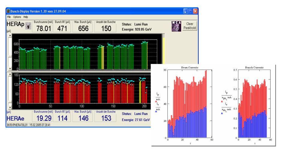
Protons: 150 bunches (3 x 50), 144 colliding, 6 pilotes (→ 3 pilotes)
