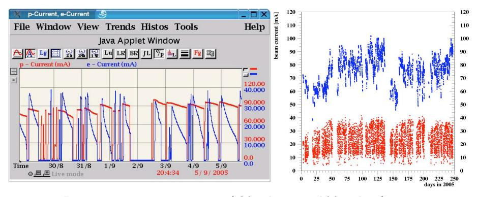
■ Proton currents up to around 90mA, up to 100 mA; electron currents 30-35 mA
