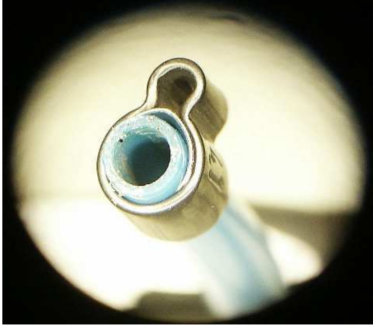
FST: leaky connection
