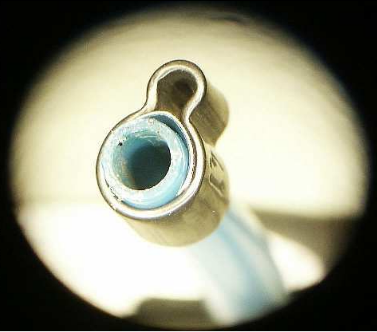
FST: leaky connection
