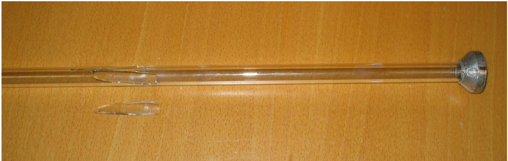
Quartzglasstube installed in June: no signal of deterioration at the moment.
