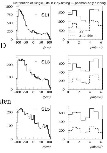
Z-vertex from tracks is at the position of the absorber (-80cm)
