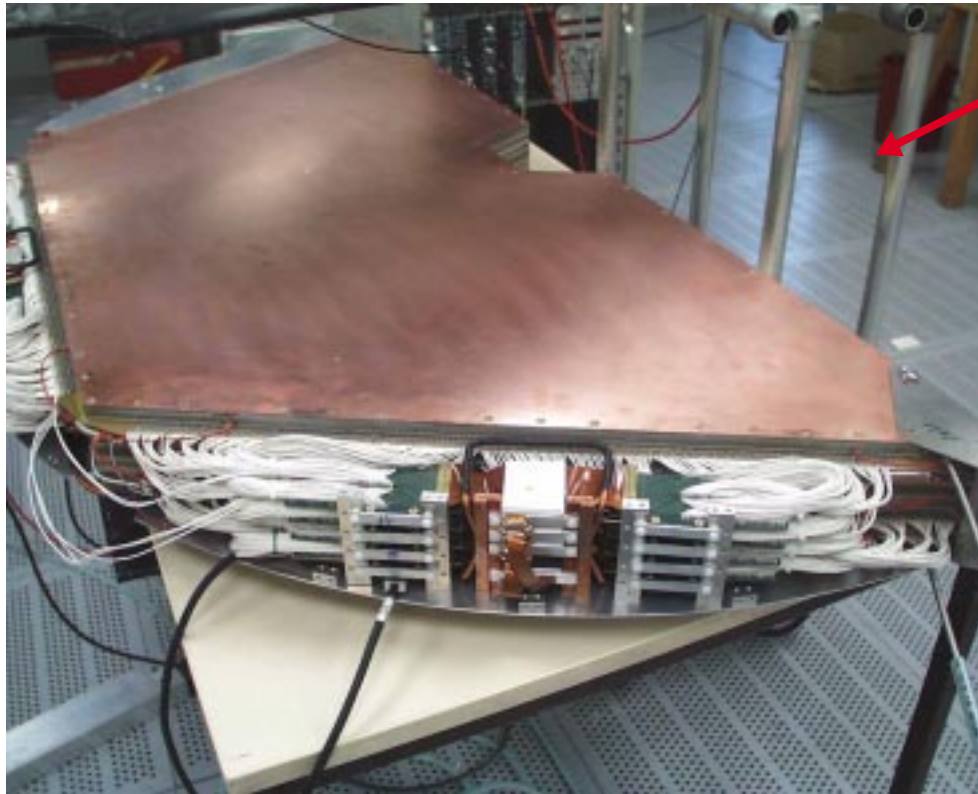
upper half of BPC on cosmic test stand
