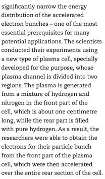
"Being more tightly bound, the electrons in the nitrogen are released a little later, and that makes them ideal for being accelerated by the plasma wave,"
