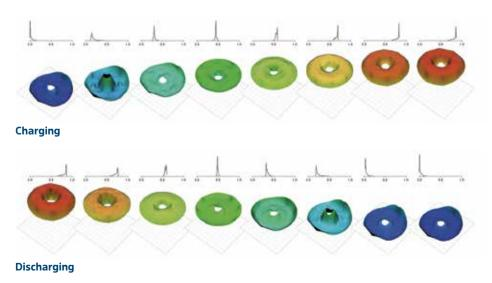
Lithium content of the anode during charging and discharging of the battery cell
