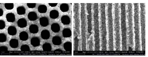
Top view (left) and crosssection (right) of the porous sponge under the electron microscope. The large cylindrical pores have a diameter of around one thousandth of a millimetre. They are separated by nanoporous walls, which are criss-crossed by pores with a diameter of only a few millionths of a millimetre.
