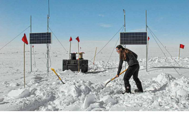
n Greenland's ice sheet, a setup unlike any other in the world will in future be listening for extremely elusive particles from space. The Radio Neutrino Observatory Greenland (RNO-G) is a pioneering project that relies on a new method of detecting very-highenergy cosmic neutrinos using radio antennas, which are being installed on and in the ice.
