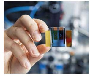
hydrogen production: The organic solar cell layer, which is only 200 nanometres (millionths of a millimetre) thin, converts light with an efficiency of almost 30 percent into electricity, which can be used directly to split water.
