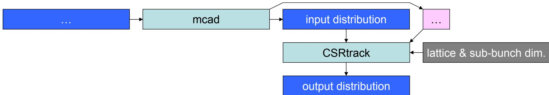
the general s2e tracking procedure is based on a 6D random distribution of equi-charged particles; such distributions are appropriate for the ‘projected’ or ‘1d’ method in CSRtrack but not for the “Green’s function method”; therefore the 6D random distribution is converted to a 4D systematic distribution of sub-bunches with individual charges; this distribution is a smooth description of essential phase space properties of the initial distribution (especially horizontal and longitudinal);
