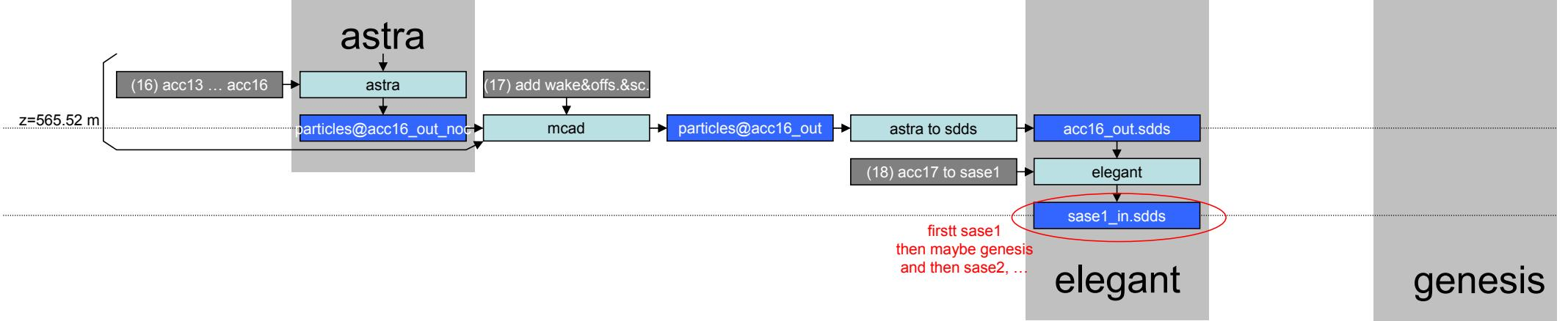
17) mcad post-processing: add centroid offset and wake of 8 TESLA modules
