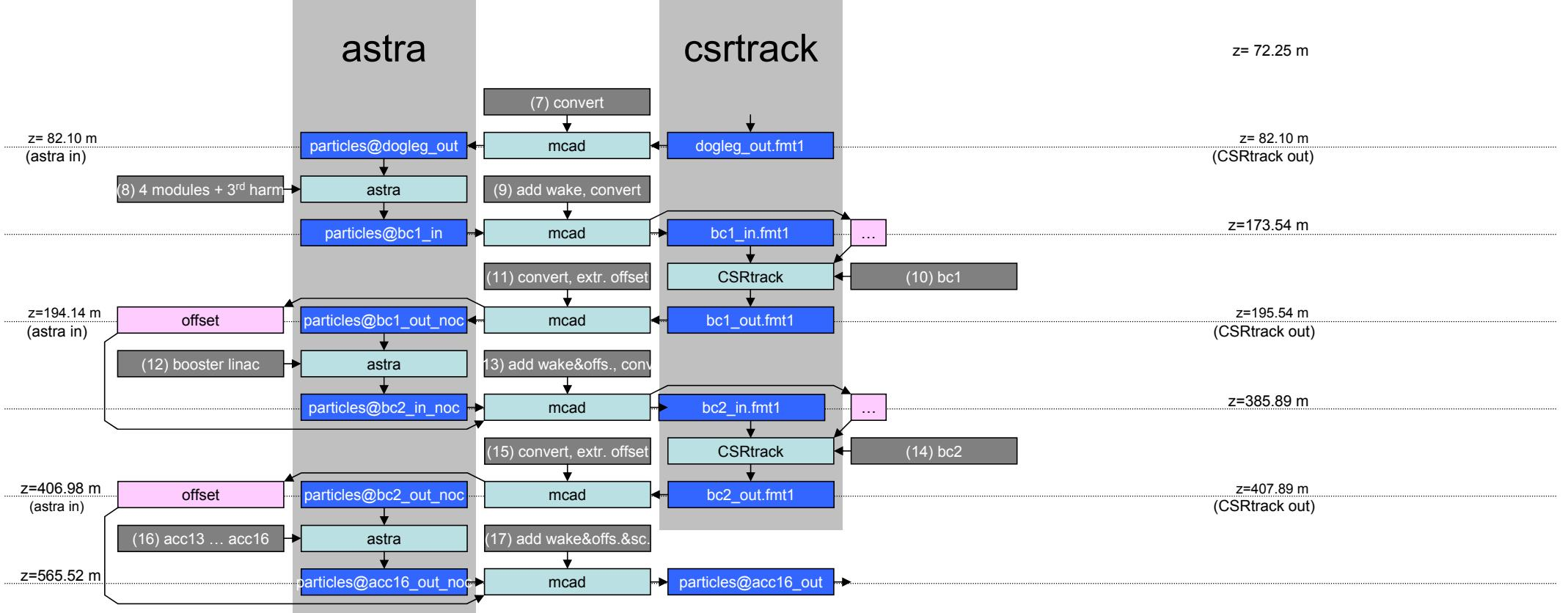
8) ASTRA calculation: 4 TESLA modules, 8 modules with 3<sup>rd</sup> harmonic rf; **the setting of amplitude and phase is quite critical** for the compression process; the values in the ASTRA input file have been optimized in several iterations;
