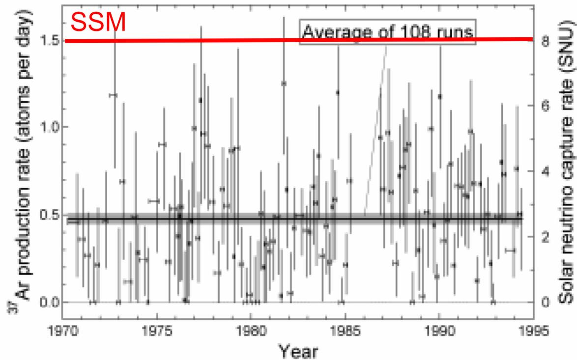
Figure 15. A summary of all of the runs made at Homestake after implementation of rise-time counting. Background has been subtracted. Over a period of 25 years, 2200 atoms of  $^{37}\text{Ar}$  were detected, corresponding to an average solar neutrino flux of 2.56 SNU. The gap in 1986 occurred when both perchloroethylene circulation pumps failed. Based on data from Cleveland *et al.* (1998).
