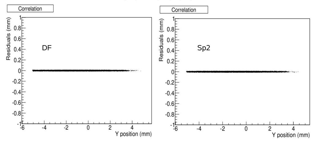
Value of the residuals as a function of the measured position on the sensors
