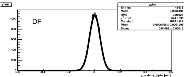
Here the sigma of the distributions is large because of the ALFA precision ( >30 um ).
