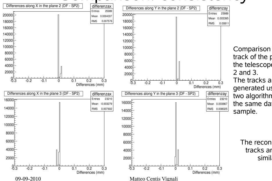
Comparison track by track of the points on the telescope planes
