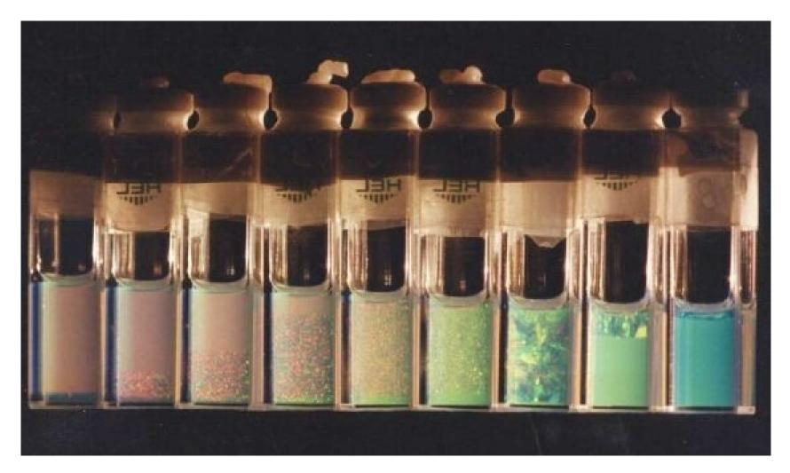
**PMMA** (in water) - poly methyl metacrylate (60 nm)
