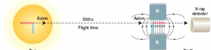
X-files. CAST "telescope" hopes to detect hypothesized particles from the sun by counting the x-rays they should produce on passing through an intense magnetic field.
