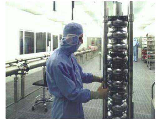
Cleanroom handling of niobium cavities
