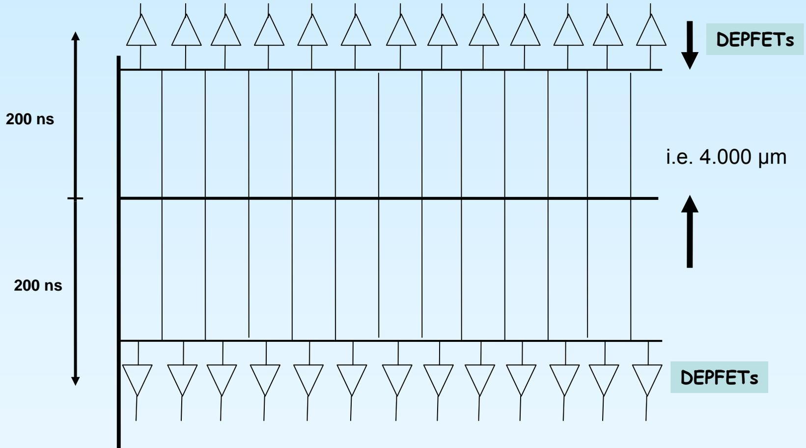
$V_{\text{max}} \approx 100 \mu\text{m/ns}$ ,  $V_{\text{exp}} \approx 20 \mu\text{m/ns}$     That means:  $\Delta t = 3 \text{ ns}$ ,  $\Delta x = 60 \mu\text{m}$
