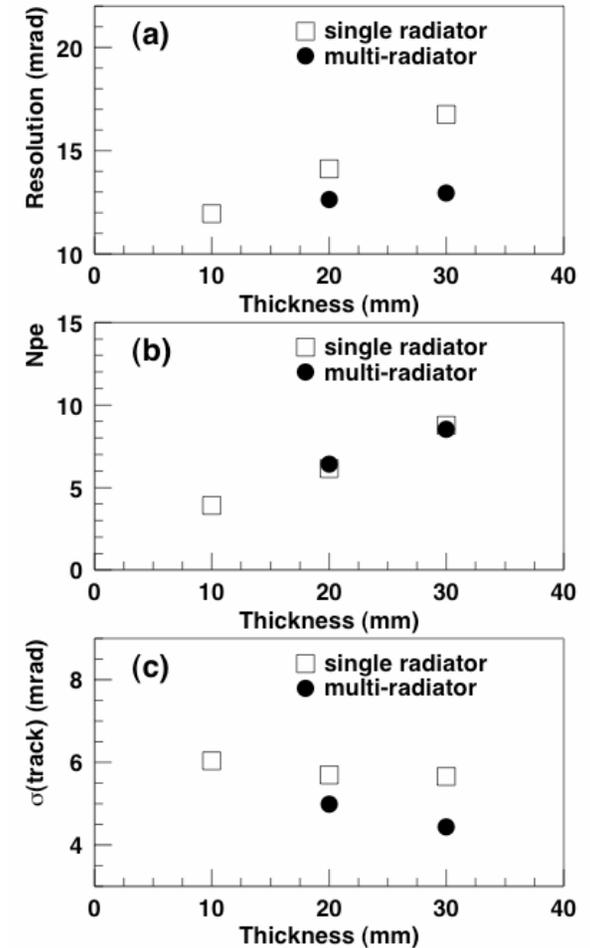
Increase Cherenkov photons without losing single angle resolution due to emission point uncertainty
