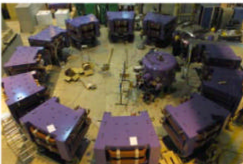
150-MeV Proton FFAG Under construction at KEK
