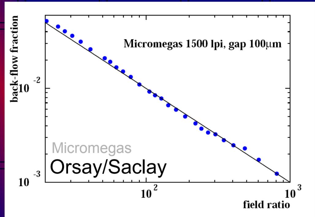
Ion backdrift  $\propto 1 / \log(\text{gain})$
