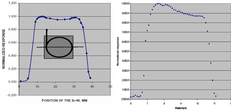
**Figure 15:** Uniformity scans for tiles with circular (left) and quarter circle grooves (right). The scan in the second case is along the diagonal perpendicular to the fibre.
