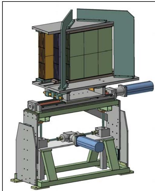
**Figure 10:** Schematic view of the support structure design.
