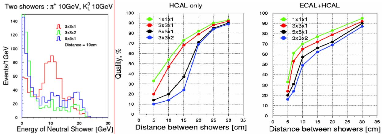
**Figure 11:** Energy of reconstructed neutral kaons (left), fraction of neutral kaons with reconstructed energy matching the true one within  $\pm 3$  standard deviations (single particle resolution), as a function of distance to next charged hadron; right: with the ECAL prototype simulated in front of the HCAL.
