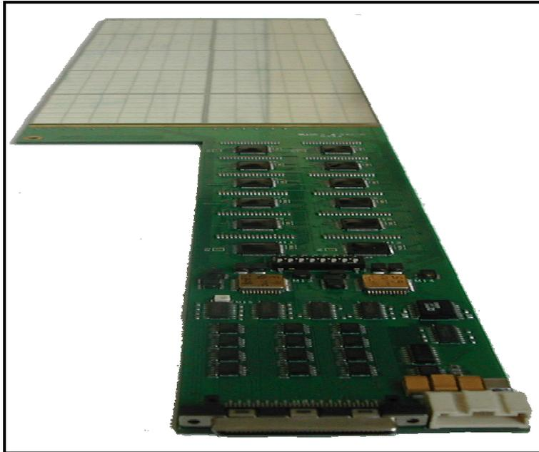
**Figure 5:** The first full size PCB with silicon wafers and the front-end electronics installed.
