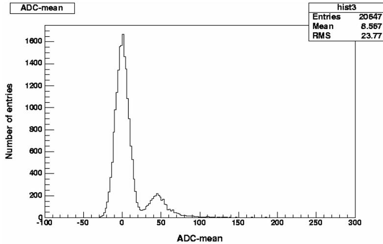
**Figure 9:** Pedestal and cosmic MIP signal on a prototype PCB with the DAQ for the prototype.
