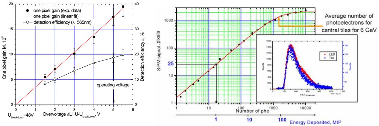
**Figure 17:** SiPM gain and efficiency vs bias voltage, response function for scintillation light signals.
