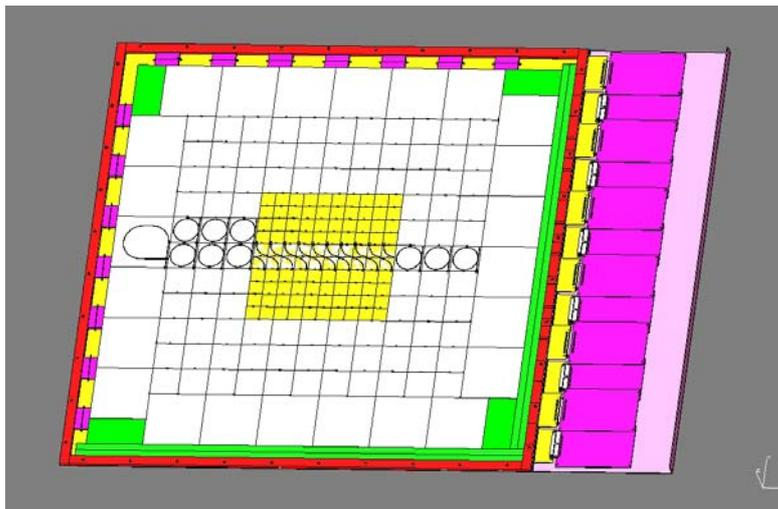
**Figure 22:** HCAL prototype cassette with front end electronics cards.
