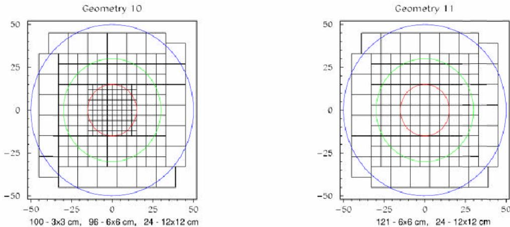
**Figure 12:** Tile geometry of prototype layer 1-30 (left) and 31-38 (right) .
