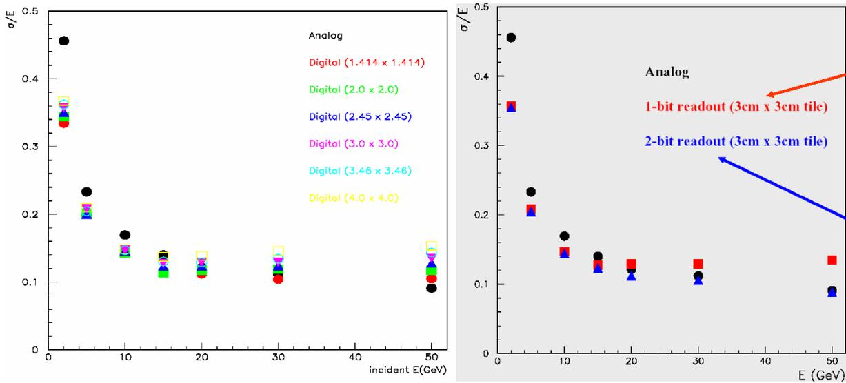
**Figure 13:** Hadron energy resolution as a function of energy for different cell sizes and numbers of thresholds.
