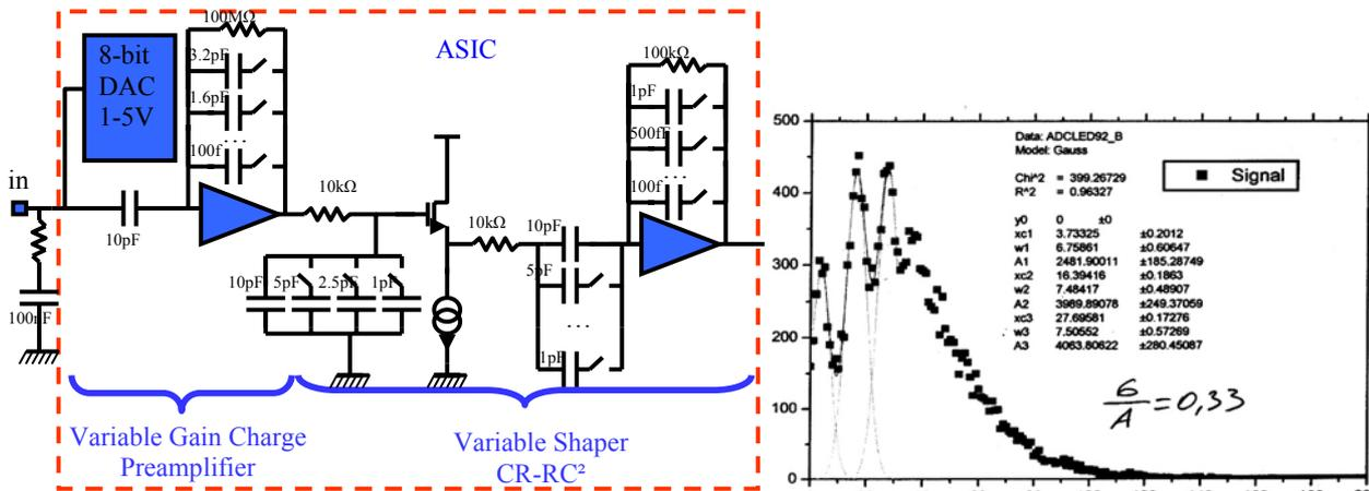
**Figure 24:** First proposal of schematics for integrated SiPM FE; measured SiPM response with slow shaping.
