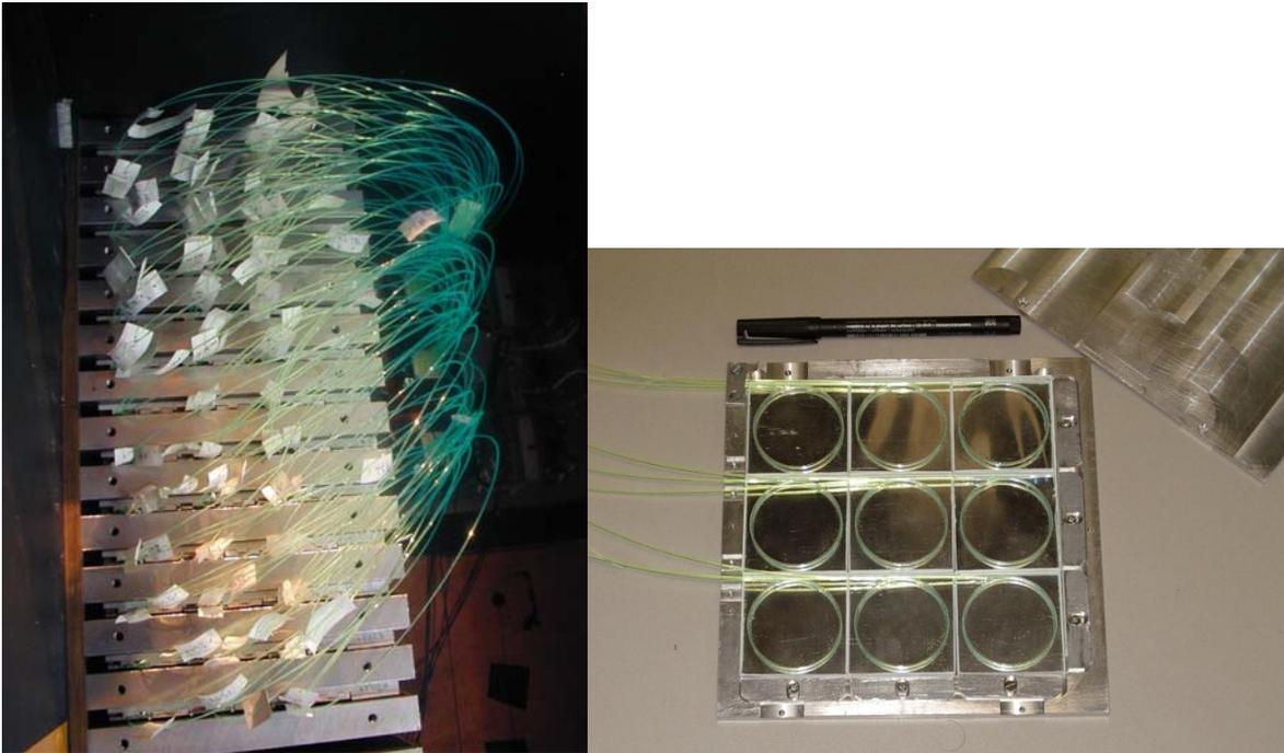
**Figure 20:** Minical structure and one active layer cassette.
