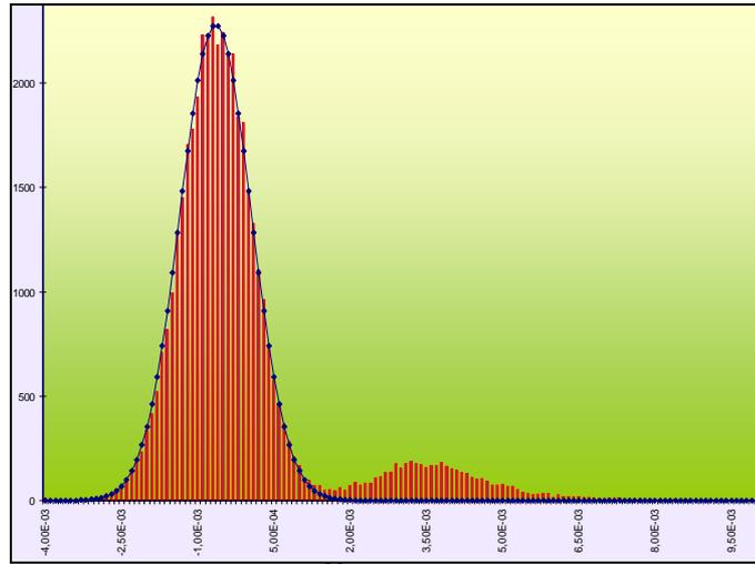
**Figure 6:** Pedestal and  $^{90}\text{Sr}$   $\beta$  signal in a prototype PCB.
