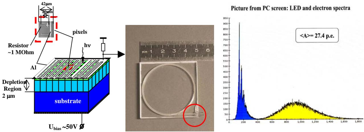
**Figure 16:** Sketch of a SiPM, SiPM mounted on a tile, pulse height spectrum from a tile irradiated by LED light and a beta source.
