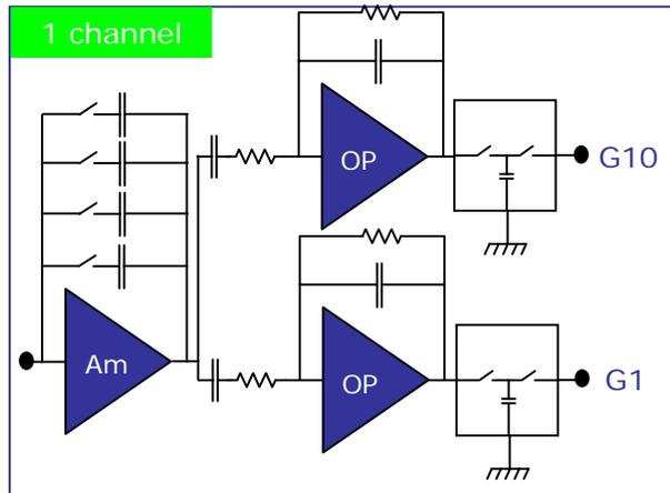
**Figure 3:** Schematic view of the VFE chip.
