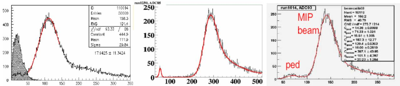
**Figure 19:** Pulse height spectra for APDs read out with a voltage sensitive preamp, a charge sensitive integrated preamp, and an integrated 18 channel preamp chip.
