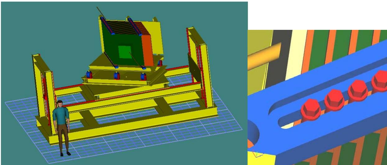
**Figure 23:** HCAL absorber stack on movable table, detail.
