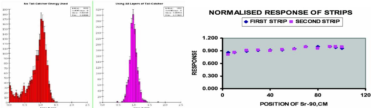
**Figure 14:** Fraction of reconstructed energy for a 50 GeV pion in the cubic metre prototype without and with a tail catcher system; uniformity scan along 1m long 5 cm wide extruded scintillator strips.
