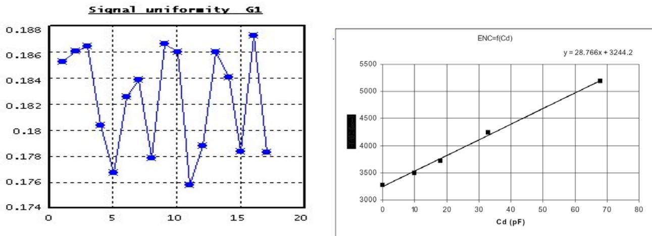
**Figure 4:** Left: signal uniformity for all 18 channels, showing it is well within 2%. Right: noise as a function of the input capacitance.
