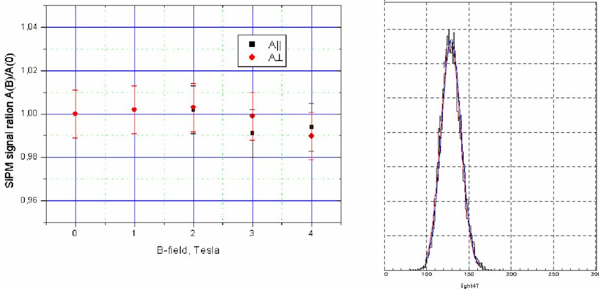
**Figure 18:** SiPM response to LED light (corresponding to about 150 pixels) vs magnetic field (left), pulse height spectrum for  $B=0$  and  $B=4T$  (right).
