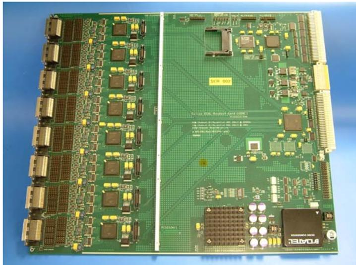
**Figure 8:** Prototype DAQ readout board.
