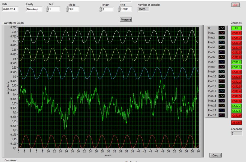
Figure 19 Environment noise, captured with OST (green) and internal noise of amplifier
