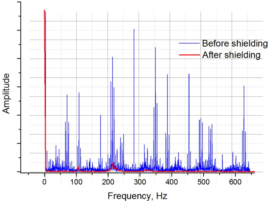
Figure 18 Noise frequency response for initial and shielded amplifier
