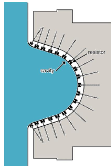
Figure 7 Thermistor positioning on the cell
