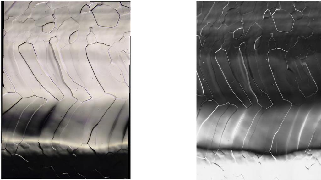
Figure 26 Microscope photography of niobium surface (left) and of its replica (right)
