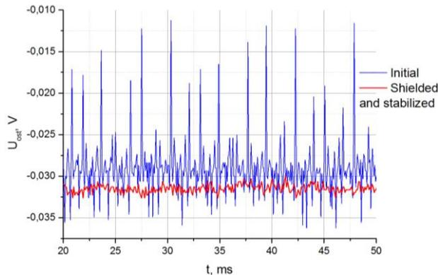
Figure 20 Noise level before and after amplifier modification
