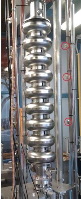
Figure 14 Assembled second sound system (OSTs in one row are circled red)
