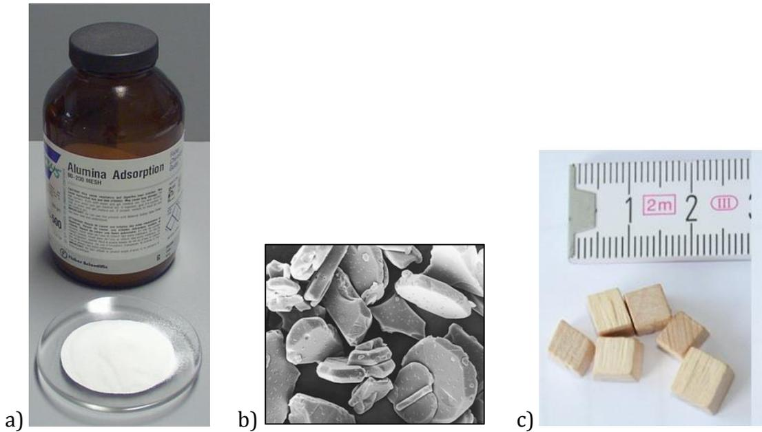
Figure 32 Photograph of alumina mesh (a), its magnified image (b) and wooden blocks (c), used for third polishing step
