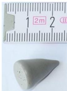
Figure 31 Photograph of plastic piece, used for second polishing step
