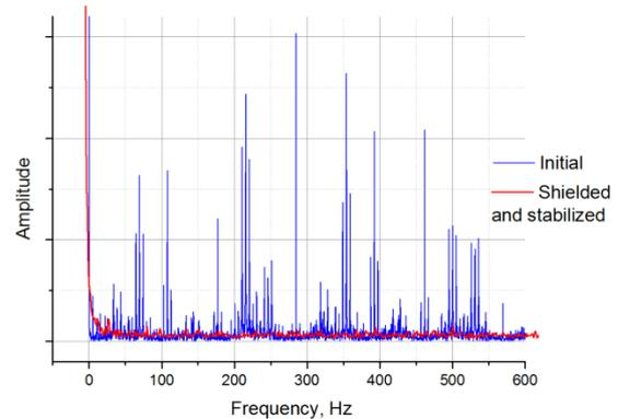
Figure 21 Noise frequency response before and after amplifier modification
