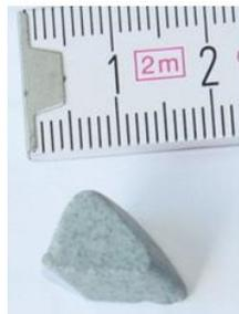
Figure 30 Photograph of stone, used for first polishing step
