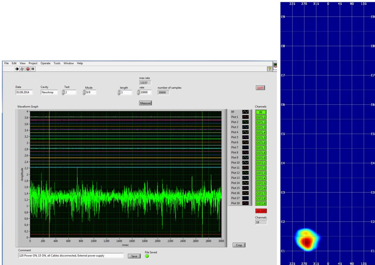
Figure 15 New DAQ software on the left, quench location output on the right
