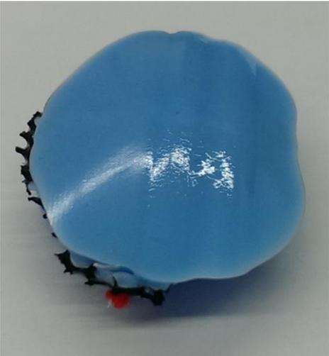
Figure 25 Silicon replica of cavity welding seam
