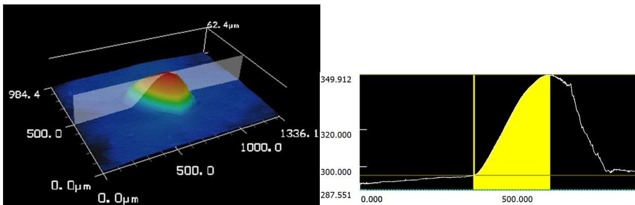
Figure 28 3D picture of surface defect (on the left) and its vertical profile (on the right)
