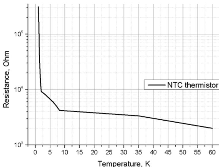
Figure 6 NTC thermistor resistance curve
