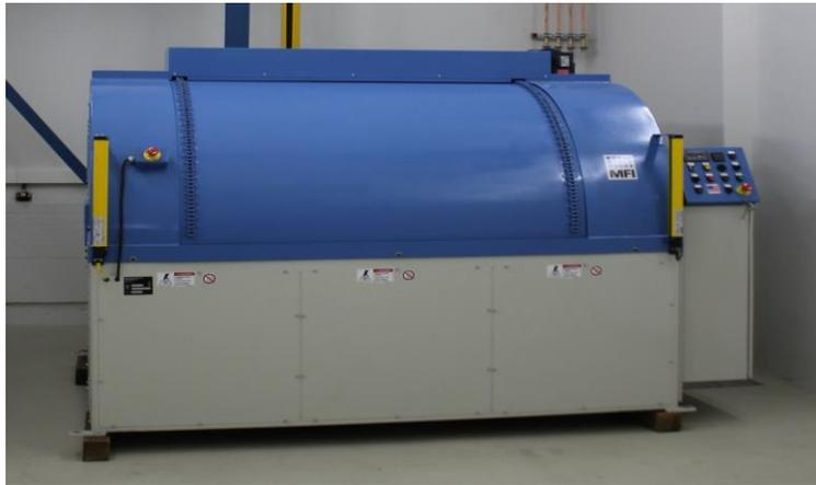
Figure 29 Centrifuge barrel for nine-cell TESLA cavity polishing
