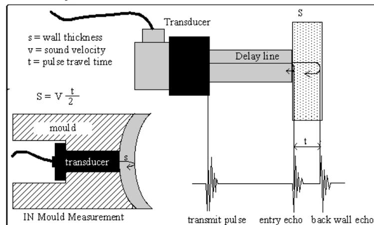
Figure 34 Ultrasound wall thickness measurement principal
