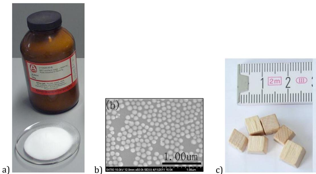
Figure 33 Photograph of silica (a), its magnified image (b) and wooden blocks (c), used for fourth polishing step
