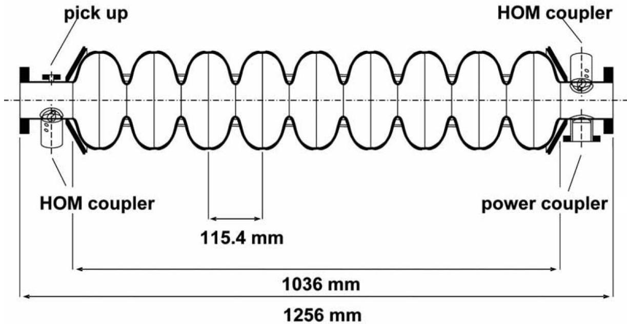
Figure 3 9-cell 1.3 GHz SRF cavity drawing (without cryogenic tank)
