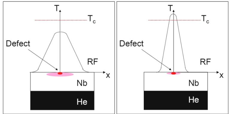
Figure 5 Quenching process
