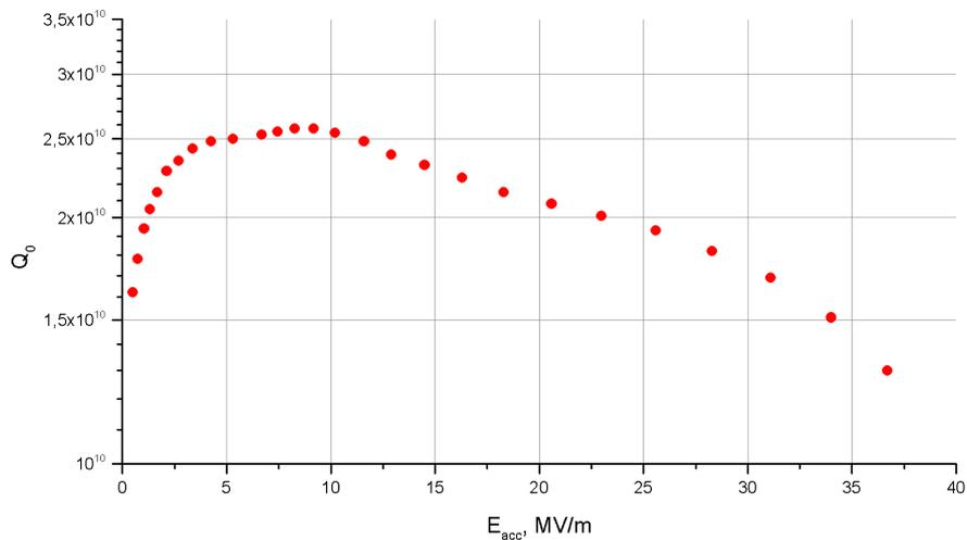
Figure 4  $Q_0$  over  $E_{acc}$  plot at 1.8K
