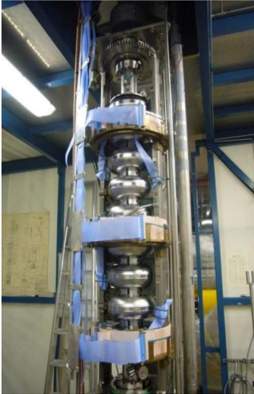
Figure 8 Assembled T-mapping system
