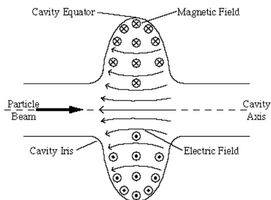
Figure 2 Field distribution in TESLA cavities (parts of cavity specified)
