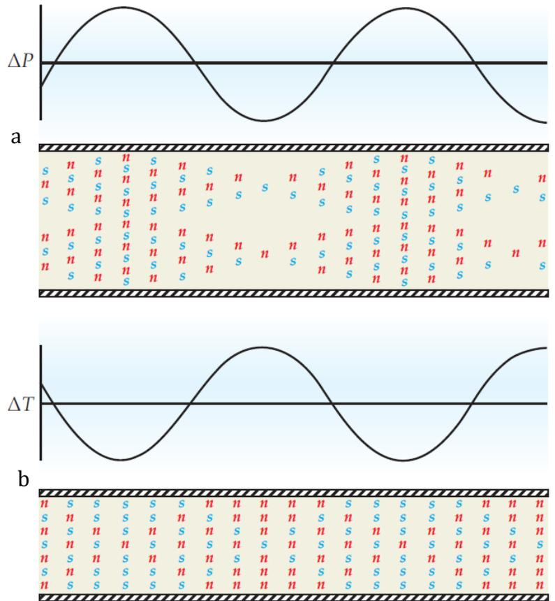
Figure 11 First (a) and second (b) sound waves and helium phases [6]
