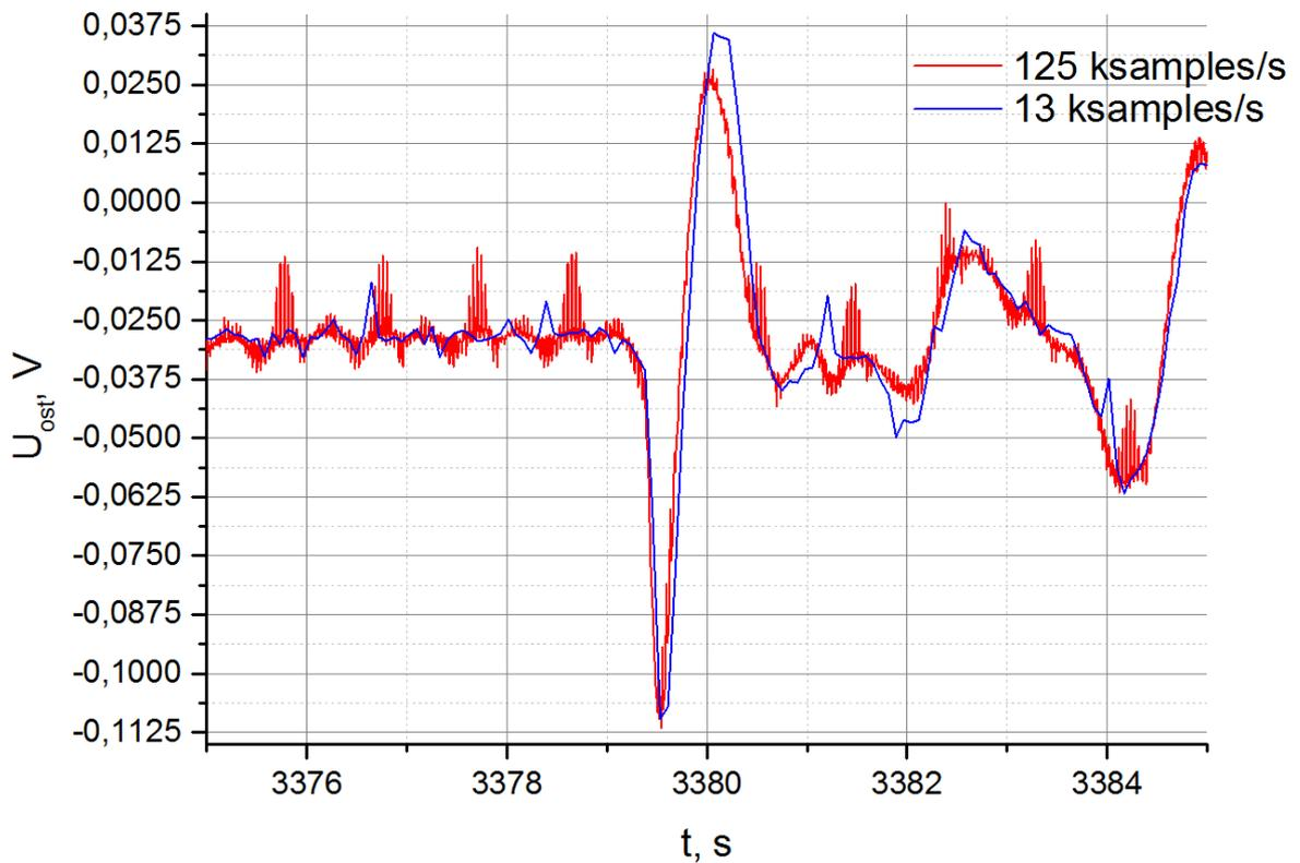
Figure 16 Signal from OST detectors converted different sample rates (13 and 125 kSamples/s)
