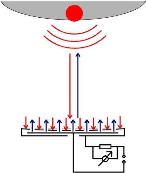
Figure 13 Principal of quench detecting using second sound wave
