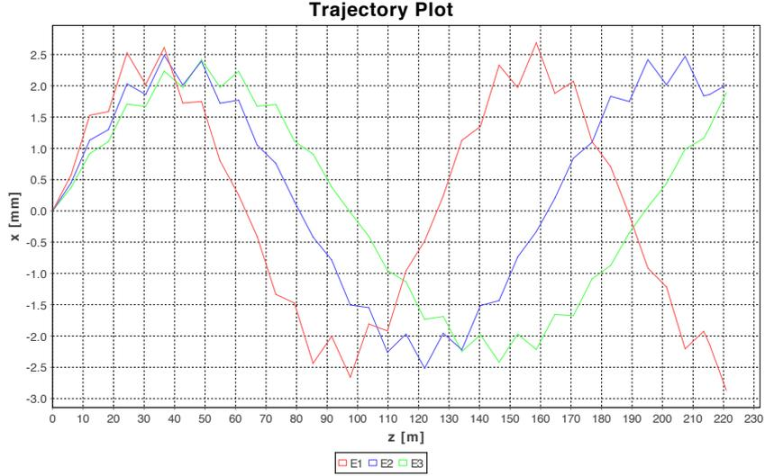
Figure 1: XZ projection of the trajectory of the beam for a one millimeter displacement of the first quadrupole in section SASE1 for energies: E1=8.0 GeV, E2=14.0 GeV, and E3=17.5 GeV
