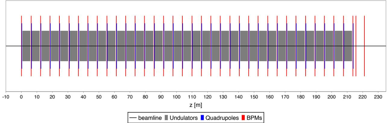
Figure 2: Schematic plot of the SASE1 section layout
