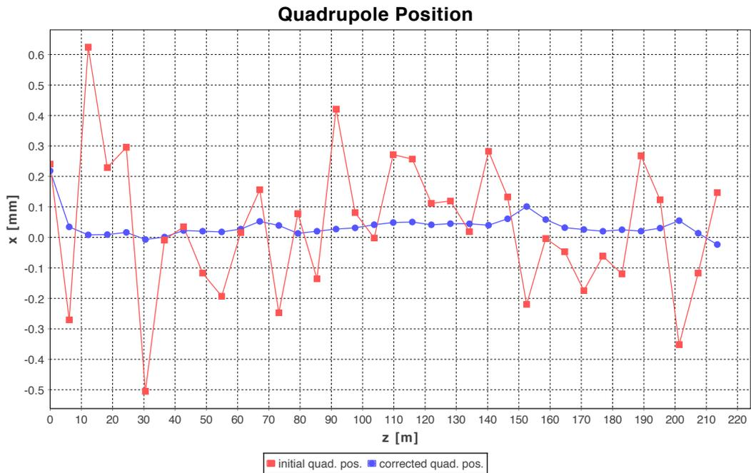
Figure 6: Quadrupole positions before and after the appliance of the method
