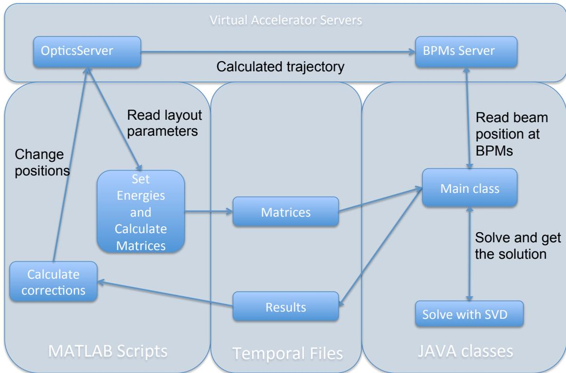
Figure 4: Scheme of connections between MATLAB scripts, Java classes and virtual accelerator servers
