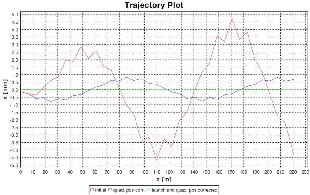
Figure 5: Trajectory of the beam before and after corrections
